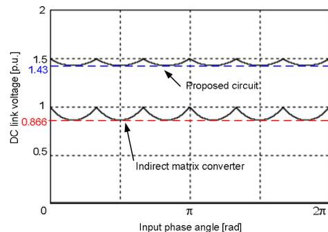
Fig. 6. DC link voltage waveform.
