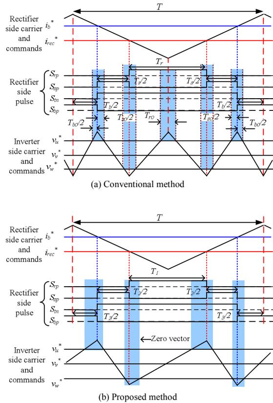
Fig. 8. Relation between inverter carrier and rectifier pulse.
