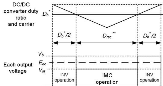
Fig. 5. The relationship between the DC link voltage and the DC/DC converter duty ratio.
