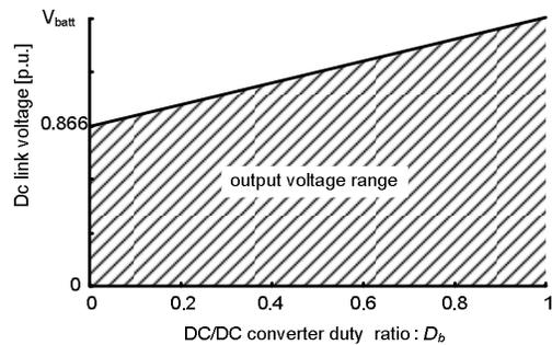
Fig. 7. Output voltage range for proposed converter.
