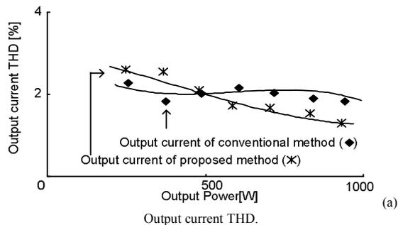
Fig. 15. THD of input and output current.
