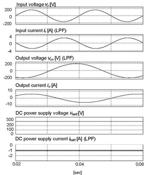
(b) Waveform when power grid regeneration, battery charge, and generating operations
