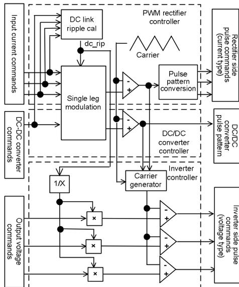
Fig. 4. Control block diagram of step-down mode.
