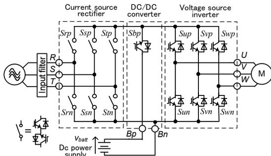
Fig. 2. Proposed circuit configuration.
