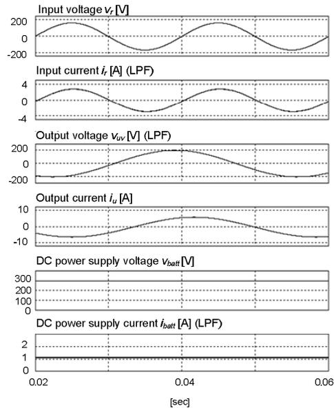
Waveform when power grid generation, battery discharge, and motoring operations
