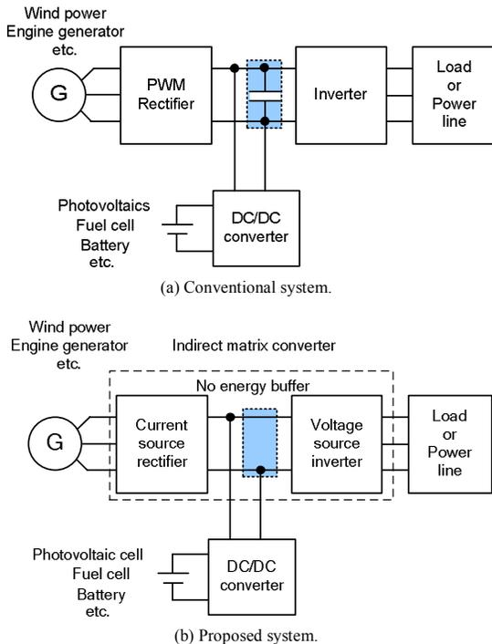
Fig. 1. Block diagrams of AC and DC power supply interface system.
