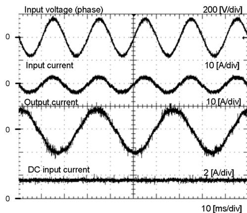
(a) Waveform when power grid regeneration, battery charge, and generating operations.
