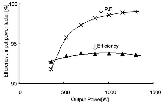
Fig. 12. Efficiency and input power factor. (IMC=indirect matrix converter; INV=inverter. )
