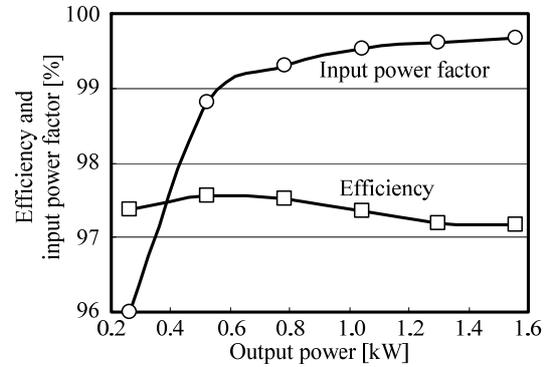
Figure 11. Input power factor and efficiency of the proposed rectifier.
