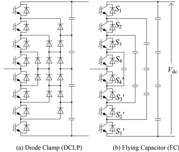
Figure 1. Conventional five-level PWM rectifier topologies (single leg).
