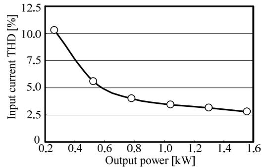
Figure 12. Input current THD of the proposed rectifier.
