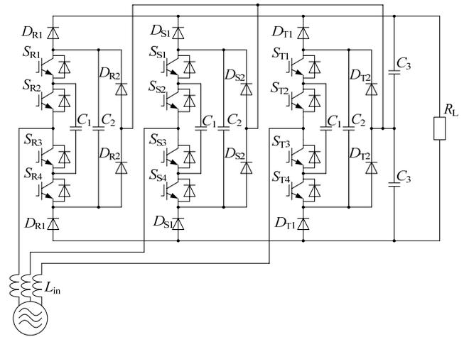
Figure 2. Proposed hybrid PWM rectifier.
