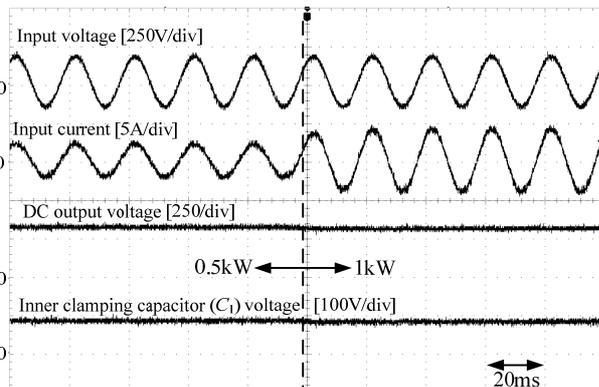
Figure 10. Experimental result of load step response.
