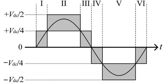
Figure 6. Rectifier input voltage waveform.
