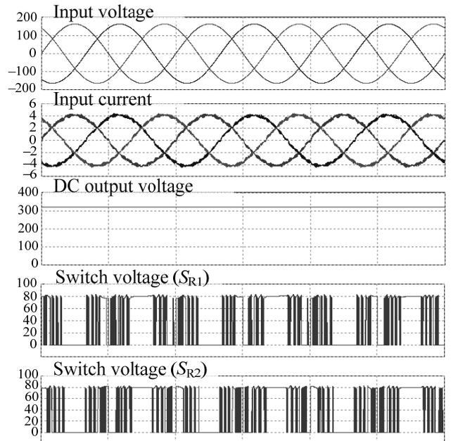
Figure 7. Simulation result of the proposed rectifier.
