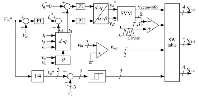
Figure 5. Control block diagram for the proposed circuit.
