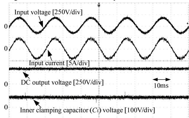
(a) Input current and DC output voltage.
