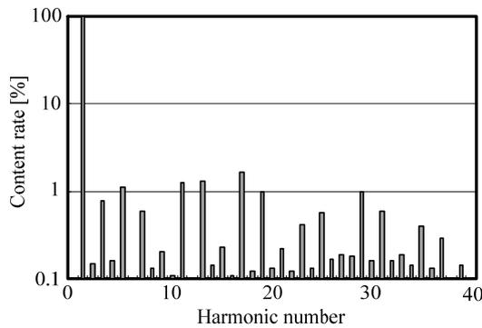
Figure 9. Harmonic current analysis at 1kW load.
