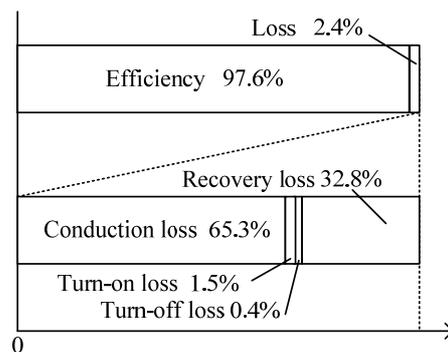
Figure 13. Loss analysis results by loss simulation at 1 kW load.
