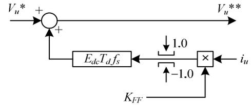
Figure 2. Conventional error voltage correction method according to the direction of motor current.
