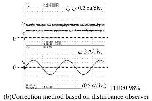
Figure 9. A Comparison of Correction performance for a disturbance observer on V/f control method.
