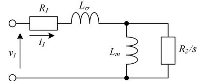
Figure 3. Equivalent circuit of induction motor.
