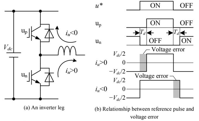
Figure 1. Relations between reference pulse and voltage error.
