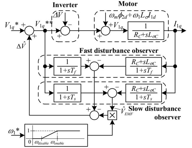
Figure 5. Block diagram of error voltage correction system for  $V/f$  control.
