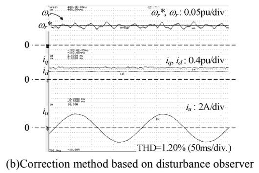
Figure 7. A Comparison of Correction performance for a disturbance observer on sensor-less vector control method.
