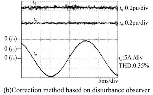
Figure 8. A Comparison of Correction performance for a disturbance observer on vector control method.
