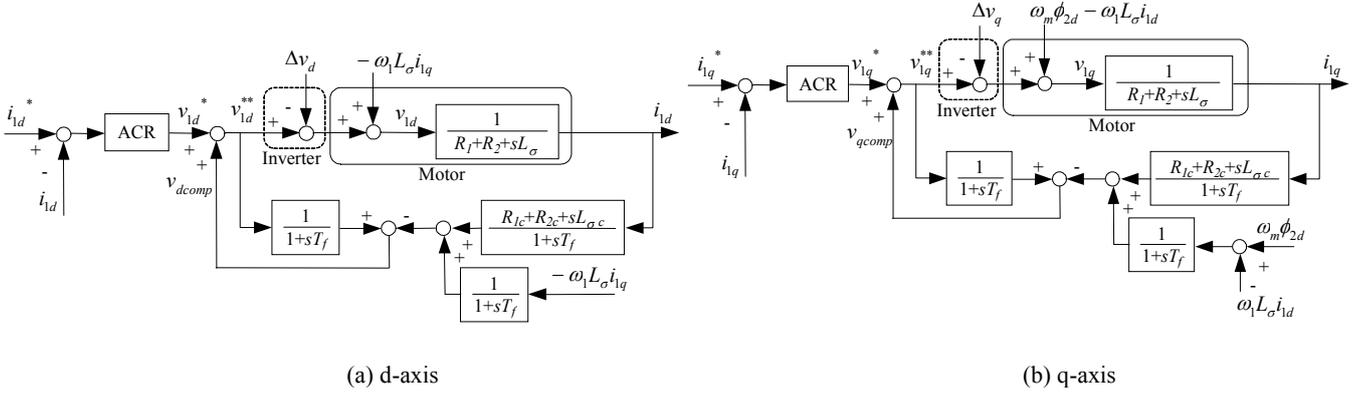
Figure 4. An error voltage correction method using a disturbance observer.
