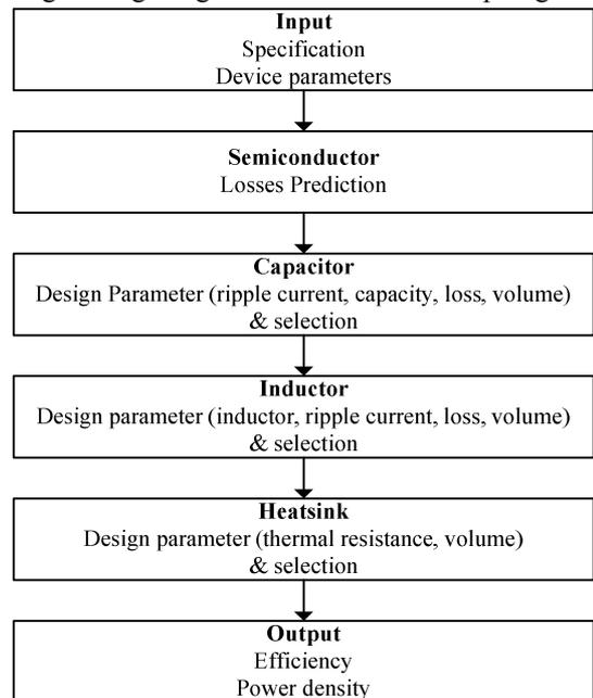
Fig. 3. Inverter design procedure.
