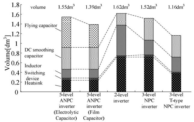
Fig. 6. Volume analysis of the inverter topologies.
