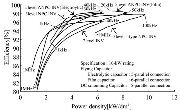
Fig. 7. Pareto front of the inverter topologies.
