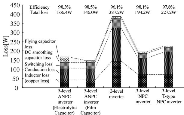
Fig. 5. Loss analysis of the inverter topologies.
