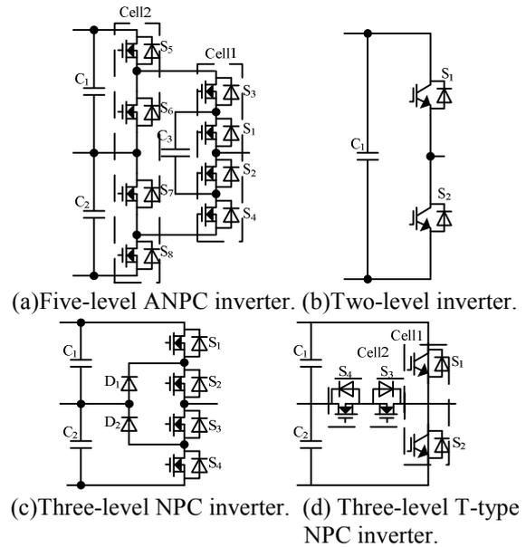
Fig. 2. Single leg multilevel converter topologies.
