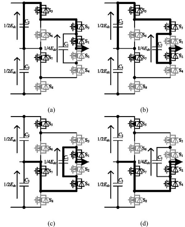
Fig. 2. Current pathway of 5-level ANPC inverter circuit topology.
