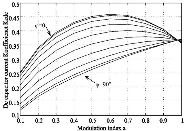
Fig.7. Current coefficient of DC smoothing capacitor.
