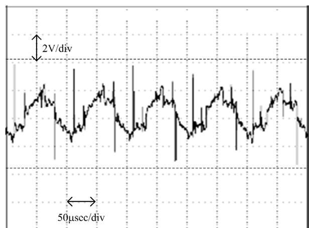
(c) Ripple voltage of the flying capacitor.
