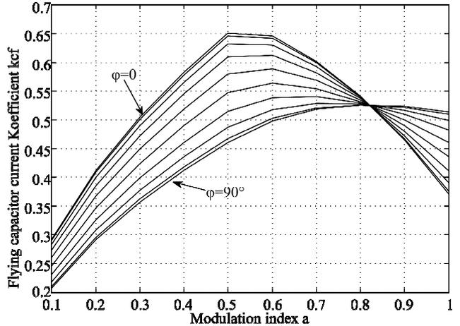
Fig.5. Current coefficient of flying capacitor.
