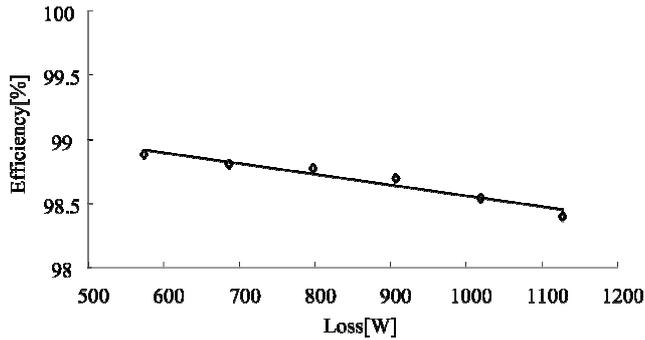
Fig.12. Efficiency of the ANPC inverter (Experimental results).
