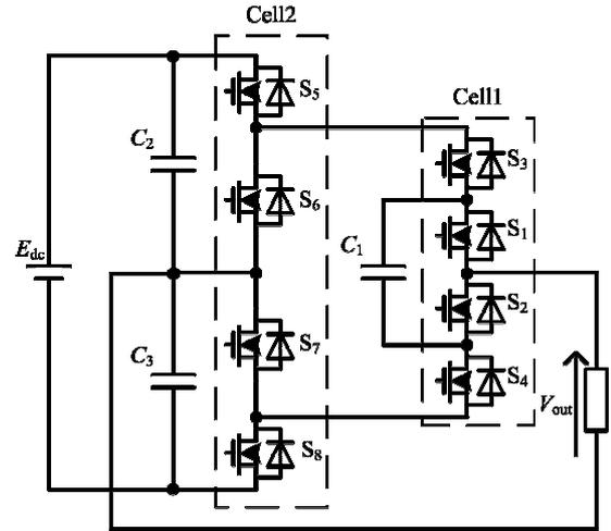
Fig. 1. Single phase 5-level ANPC inverter circuit topology.
