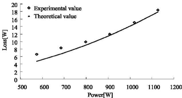
Fig.8 Loss of the ANPC inverter.
