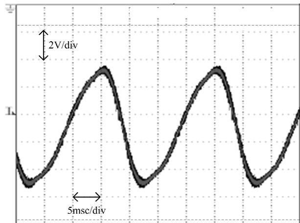
(b) Ripple voltage of the DC smoothing capacitor
