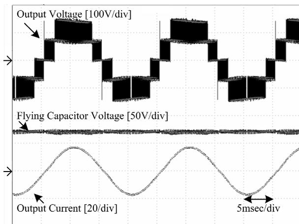
Fig.10. Experimental waveform of the ANPC inverter.
