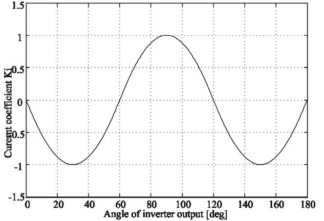
Fig.6 Relationship of angle of inverter output and current coefficient.
