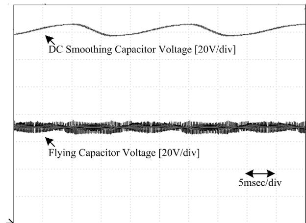
(a) Voltage waveform of the capacitors.
