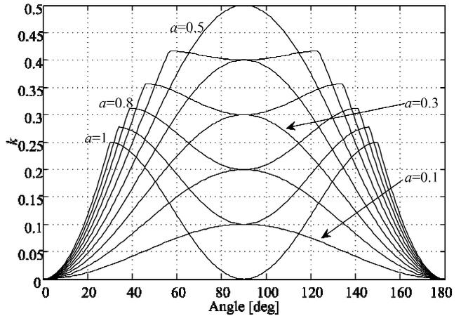
Fig.4. Relationship of output phase and voltage coefficient  $k$ .
