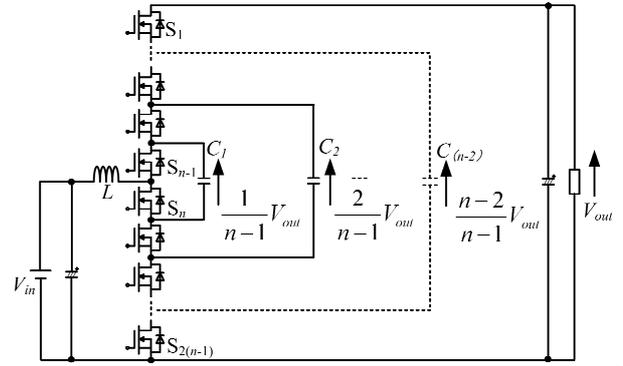
Fig. 16.  $n$ -level switched capacitor converter.
