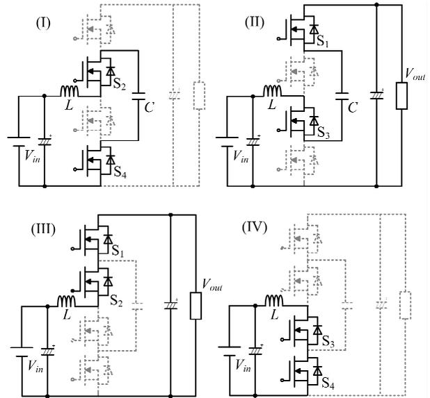
Fig. 5. Operation mode of 3 level SCC with input reactor.
