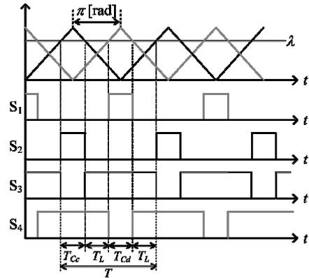
Fig. 4. Switching pattern of the 3-level SCC.
