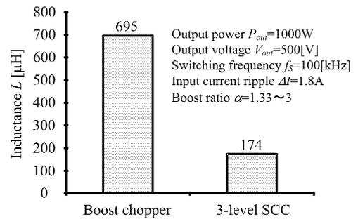
Fig. 7. Comparing of inductance between a conventional boost chopper and a proposed 3-level SCC.
