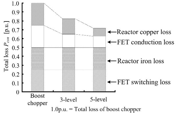
Fig. 21. Reduction of total loss by multi-level.
