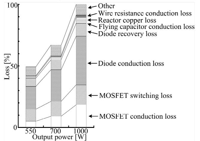
Fig. 14. Loss separation of output load characteristics.
