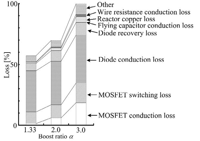
Fig. 15. Loss separation of boost ratio characteristics.
