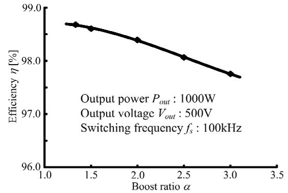
Fig. 13. Boost ratio characteristics.
