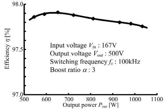
Fig. 12. Output load characteristics.
