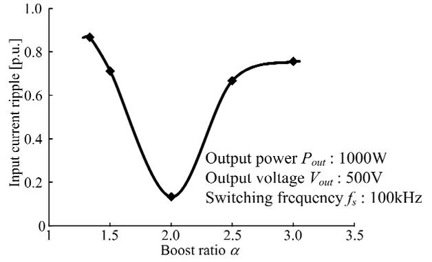
Fig. 11. Input current ripple characteristics.
