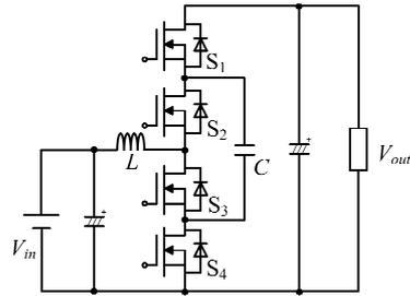
Fig. 3. 3-level output voltage control SCC.
