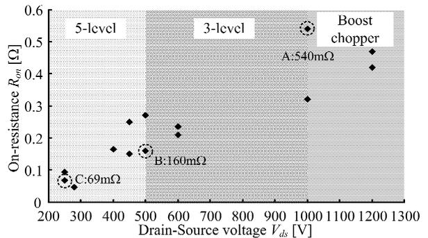
Fig. 18. Drain-source voltage v.s. on-resistance.
