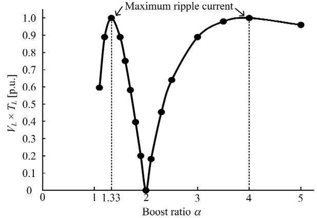
Fig. 6. Relation between the volte time products and boost ratio in the proposed circuit.
