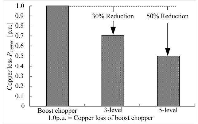
Fig. 20 Comparing to the copper loss by multi-level.
