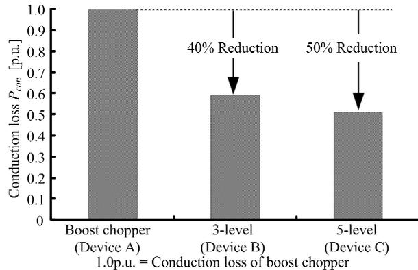
Fig. 19. Comparing to the conduction loss by multi-level.
