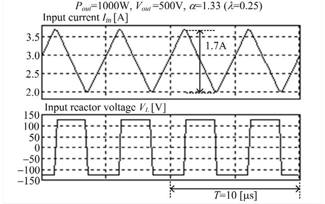
Fig. 8. Operation waveforms by simulation at the boost ratio of 1.33.
