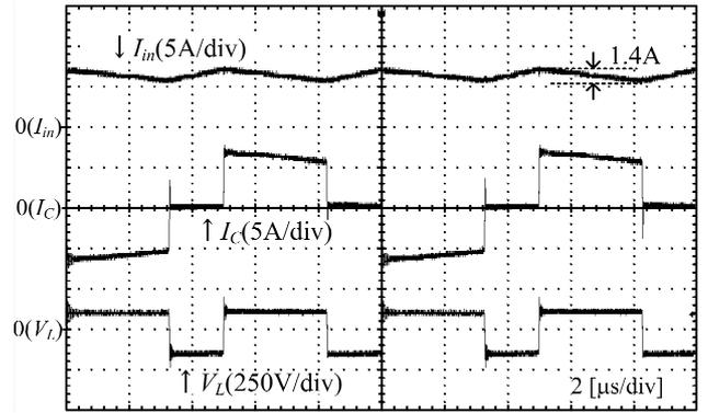
Fig. 10. Operation waveforms (3-times boost and 1000W).
