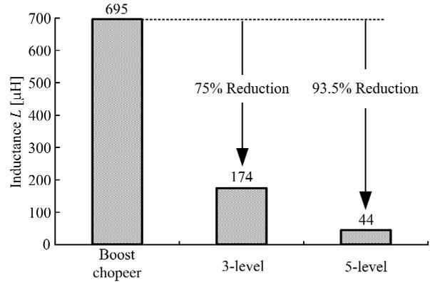
Fig. 17. Relationship between the number of level and inductance.
