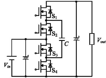
Fig. 1. Boost type 3 level switched capacitor converter.
