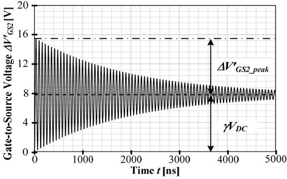
Fig. 8 The  $\Delta V'_{GS2}$  waveform derived from a calculation formula.
