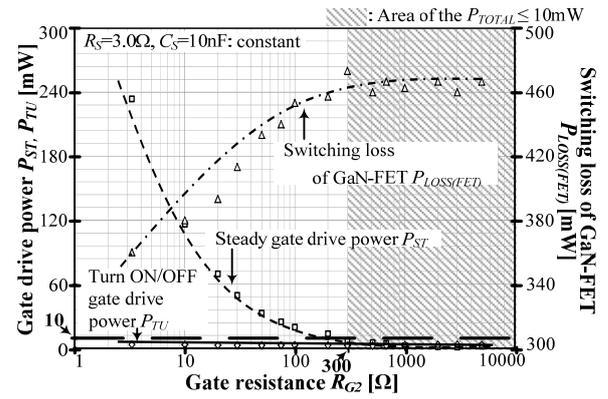
Fig. 2. Relationship between the gate resistance and the power consumption.  $R_{G2}$  is a variable parameter. ( $R_S=3.0\Omega$ ,  $C_S=10nF$ : constant)
