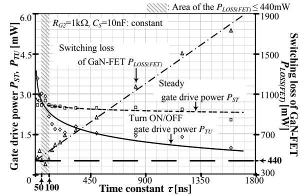
Fig. 3. Relationship between the time constant and the power consumption.  $R_S$  is a variable parameter. ( $R_{G2}=1k\Omega$ ,  $C_S=10nF$ : constant)
