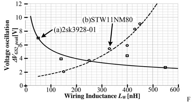
Fig. 11. The difference in the characteristics by switching devices.
