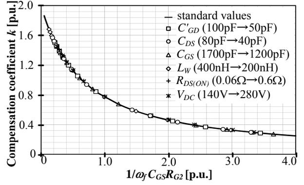
Fig. 9. Compensation coefficient calculation curve.
