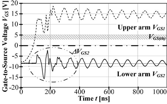
Fig. 6. The voltage oscillation of source-to-gate voltage.
