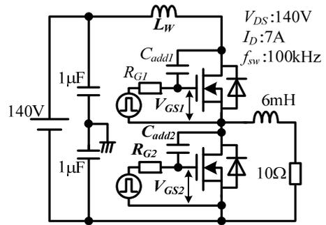
Fig. 5. Experimental and simulation circuit composition.
