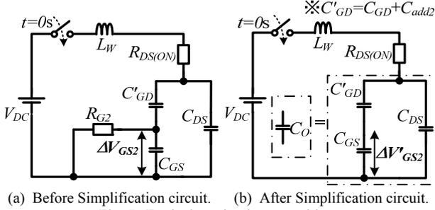
(a) Before Simplification circuit. (b) After Simplification circuit.
