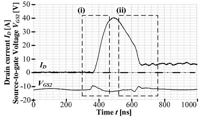
Fig. 14. A drain current  $I_D$  waveform and a source-to-gate voltage  $V_{GS2}$  waveform.
