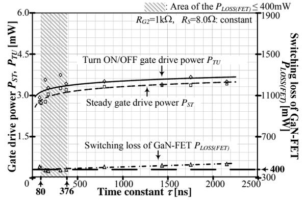
Fig. 4. Relationship between the time constant and the power consumption.  $C_S$  is a variable parameter. ( $R_{G2}=1k\Omega$ ,  $R_S=8.0\Omega$ : constant)
