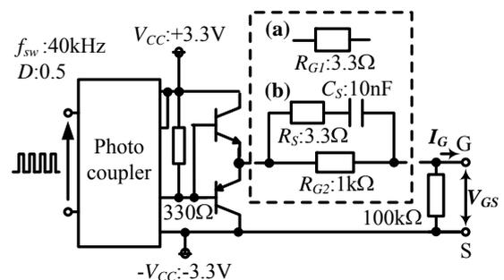
Fig. 1. Configurations (a) and (b) of the gate drive circuit.
