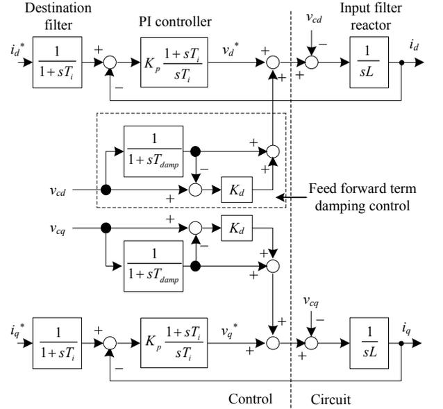
Fig. 7. Transfer function block diagram in ACR to control the input current of the matrix converter.
