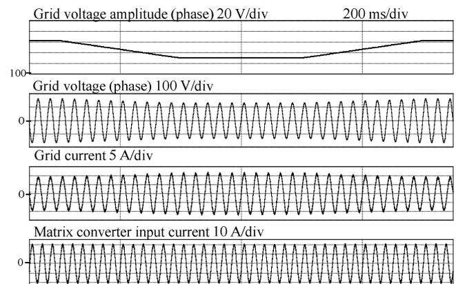
Fig. 12. Operation waveforms of the proposed system in period of the fluctuation of the power grid voltage.
