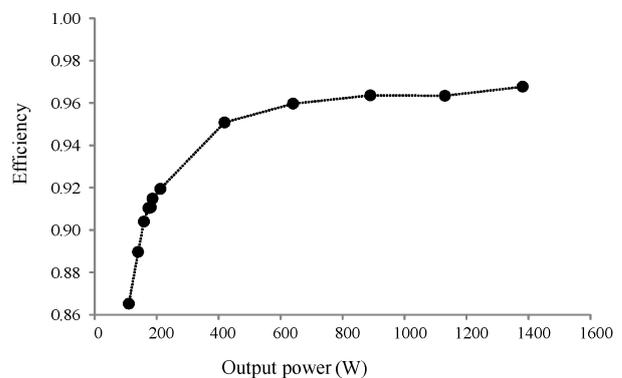
Fig. 14. Efficiency characteristics with experiment.
