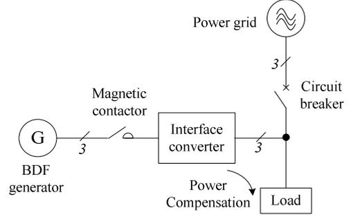
Fig. 1. Configuration diagram of an interconnection system using an interface converter for a smart grid.
