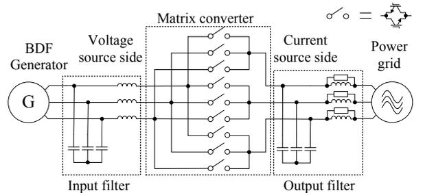
Fig. 3. Configuration diagram of the proposed power grid connected system using a matrix converter.
