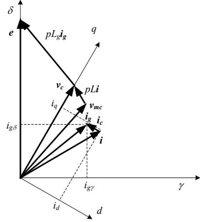
Fig. 4. Relationship among the voltages and the currents on the generator side with dq axis based on the terminal voltage and  $\gamma\delta$  axis based on the back electromotive force of the generator.
