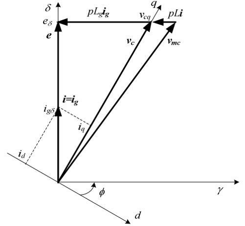
Fig. 6 The vector diagram on the generator side when the generator current vector and the voltage vector of the back electromotive force of the generator are in the same phase.
