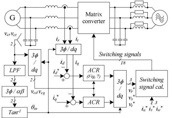
Fig. 5. Control block diagram of the proposed interface system between an engine generator and the power grid.
