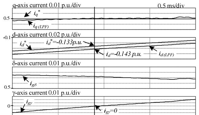
Fig. 9 Relationship between a zero point of the  $\gamma$ -axis current and the input current command of the matrix converter.
