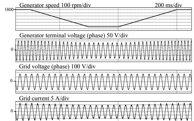
Fig. 11. Operation waveforms of the proposed system including no distortion in the period of the generator frequency fluctuation.
