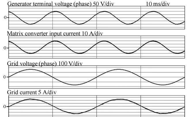
Fig. 8. Operation waveforms of the matrix converter in the proposed system at steady state in simulation.
