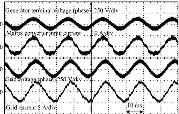
Fig. 13. Operation waveforms of the proposed system at steady state with an experiment.
