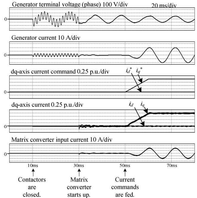
Fig. 10. Voltage and current waveforms on the generator side in the starting sequence of the proposed interface system.
