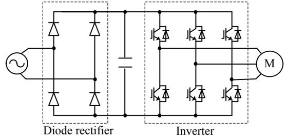
(a) Diode rectifier and inverter type.
