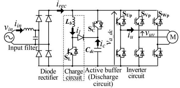
Fig. 3. Proposed circuit configuration.
