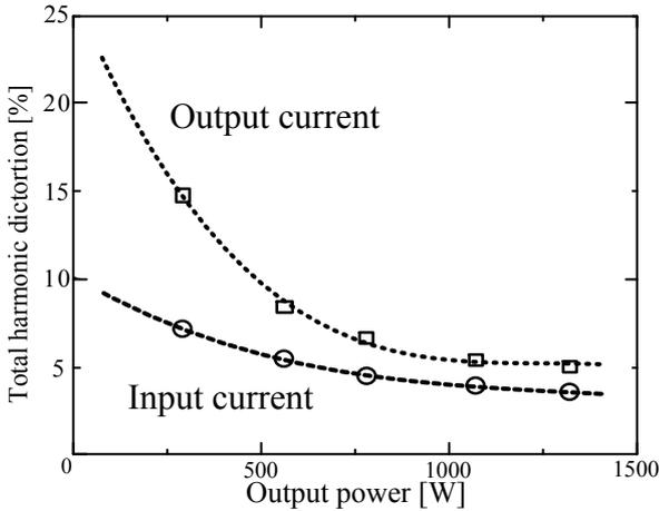
Fig. 12. THD of the input and output current.
