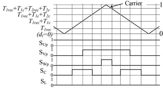
(c) Discharge period (switch  $S_C$  hard-switching method).
