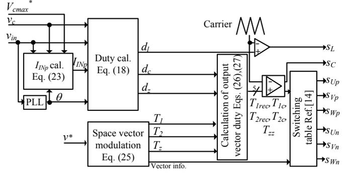
Fig. 7. Control block diagram.
