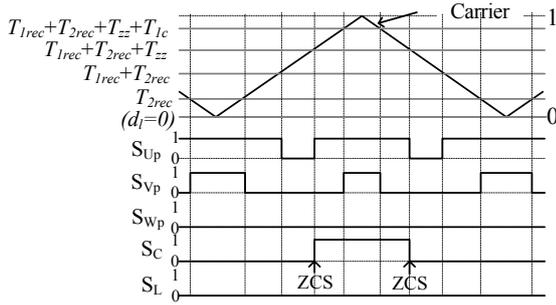
(b) Discharge period (switch  $S_C$  soft-switching method).
