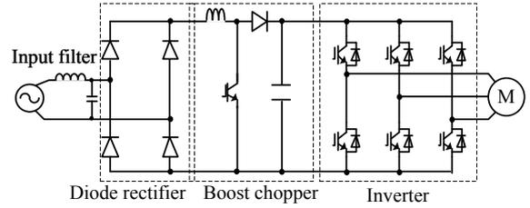
(b) Diode rectifier, boost chopper and inverter type.
