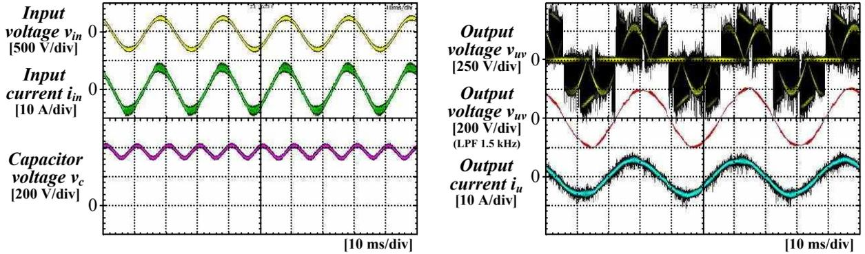
(a) Input and capacitor voltage waveforms.
