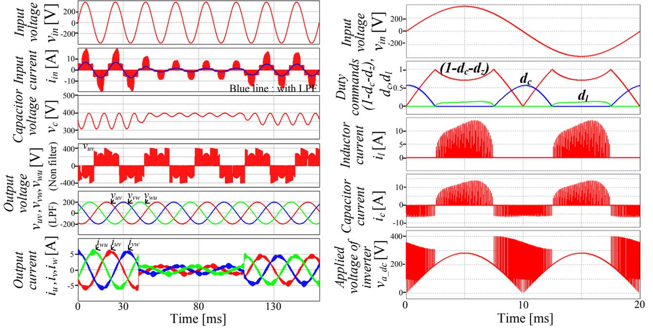
(a) Relationship among input/output waveforms and capacitor voltage.
