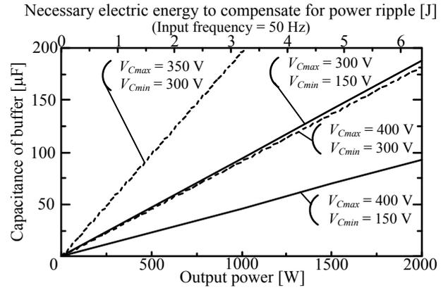
Fig. 8. Relationship between necessary electric energy or necessary capacitor and output power when input frequency is 50 Hz.
