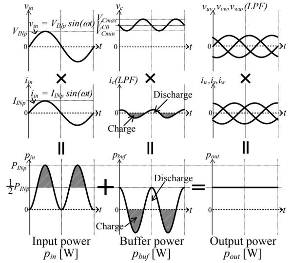
Fig. 4. Compensation principle of power ripple.
