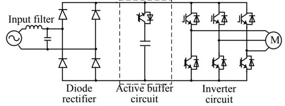
Fig. 2. Previous single-to-three-phase converter with active buffer circuit.
