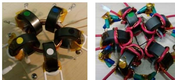
(a) Secondary wiring through cores. (b) Bifilar wound transformer.
