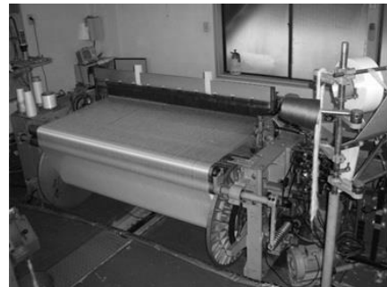
Fig. 2 The weaving machine (JW-832C).
