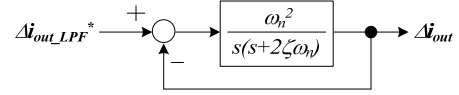
Fig. 5. Approximate block model between \Delta i_{out\_LPF}^* and \Delta i_{out} without the output damping control to simplify the design procedure. The transfer function of this block diagram becomes the standard form of the second order system.
