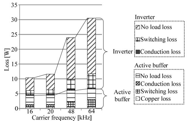
Fig.14 Converter loss analysis results.
