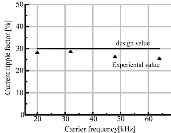
Fig. 11 Buffer inductor current ripple factor.
