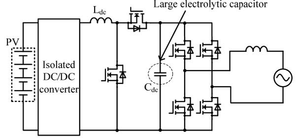
Fig.1 Conventional circuit for PV micro inverter.
