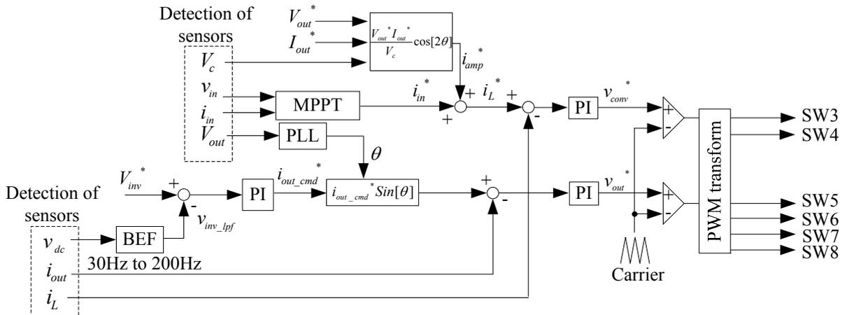
Fig.4 Control block diagram for the proposed circuit.
