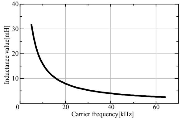
Fig.7 Relationship between buffer inductance and carrier frequency.
