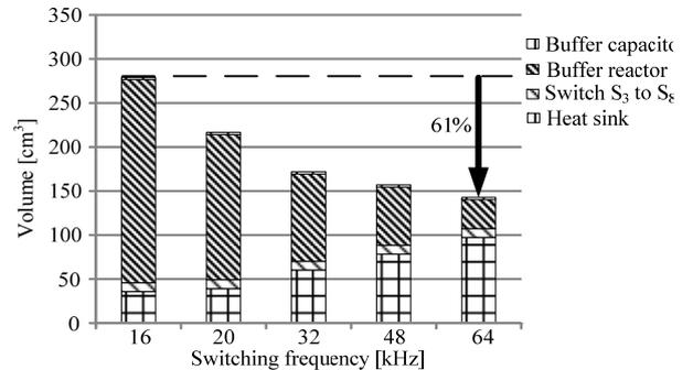
(b) Volume comparison when the switching frequency increase to 64kHz.
