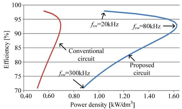
Fig.17 Pareto front curve of the conventional circuit and proposed circuit.
