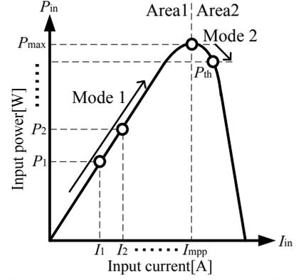
Fig.5. Behavior of the operation point in MPPT.
