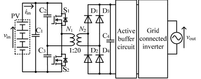
(a) Isolated resonance DC/DC converter.
