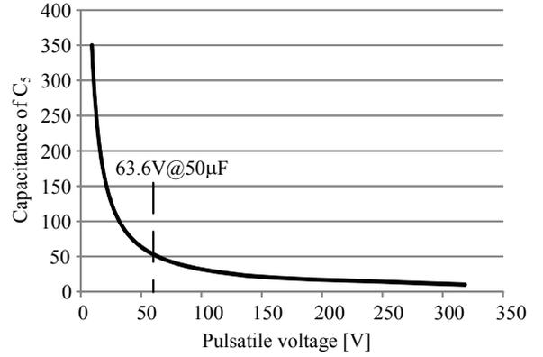
Fig.6 Relationship between the pulsatile voltage and capacitance of  $C_5$ .
