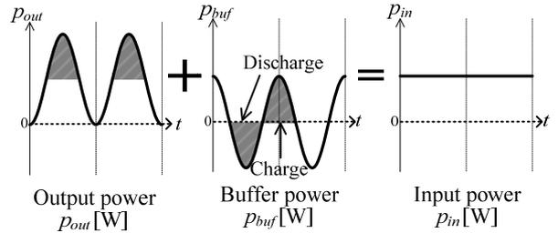
Fig.3 Compensation principle of the power ripple with active buffer.
