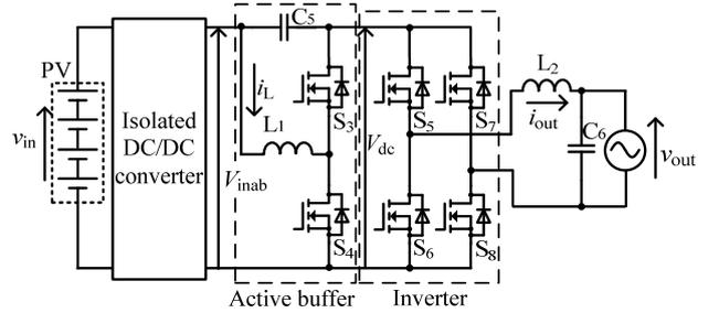
(b) Active buffer, inverter circuit.
