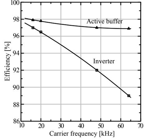
Fig.15 Relationship between the carrier frequency and efficiency.
