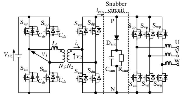
Fig.1. DC-AC converter with indirect matrix converter.
