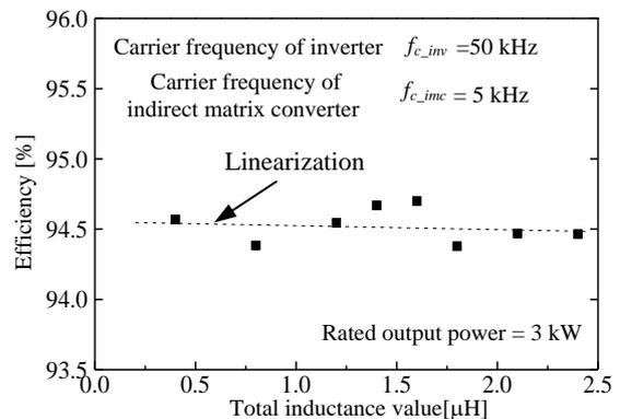
Fig.4. Comparison of efficiency at rated power.
