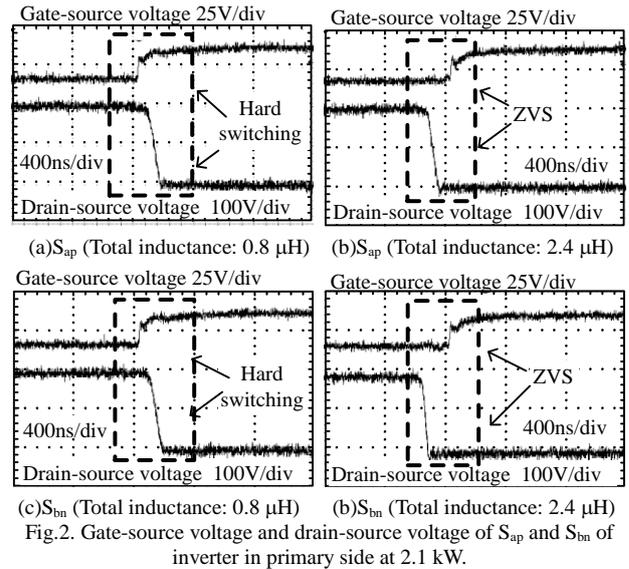
Fig.2. Gate-source voltage and drain-source voltage of  $S_{ap}$  and  $S_{bn}$  of inverter in primary side at 2.1 kW.
