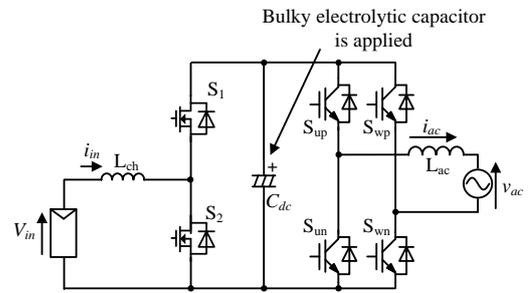
Fig.1. General configuration for DC to single-phase AC grid connection system. This circuit has a large electrolytic capacitor  $C_{dc}$  on the DC link part.  $C_{dc}$  is usually used the bulky electrolytic capacitor.
