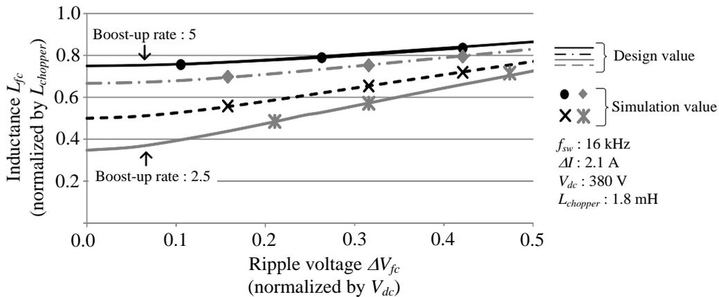
Fig.8 Relationship between the ripple voltage of the flying capacitor and inductance of the boost-up inductor.
