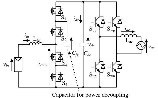
Fig.3. Proposed circuit using the flying capacitor DC-DC converter topology. This circuit use the flying capacitor  $C_{fc}$  in order to compensate the single-phase power fluctuation. Thus, the additional component is not needed.
