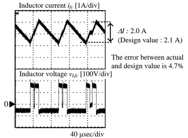
Fig.14 Estimation of the ripple current of the boost-up inductor.
