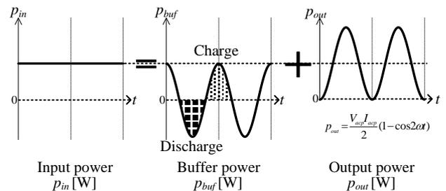
Fig.4. Compensation principle of the single-phase power fluctuation. The power ripple that contains frequency twice of the grid frequency appears at DC link voltage. In order to compensate the power fluctuation at input DC side, buffer power  $p_{buf}$  is fluctuated by flying capacitor  $C_{fc}$ .
