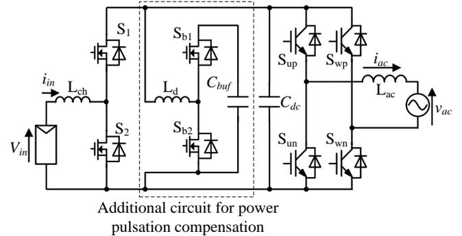
Fig.2 Power conditioner system using the conventional active power decoupling method. This circuit needs an additional inductor and switching devices. It cause low efficiency and large circuit volume.
