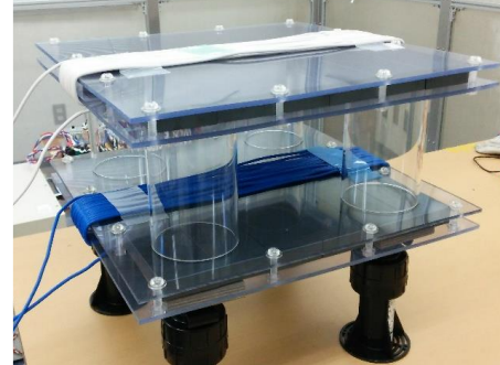
Fig. 7. Transmission Coils for 3-kW Prototype.
