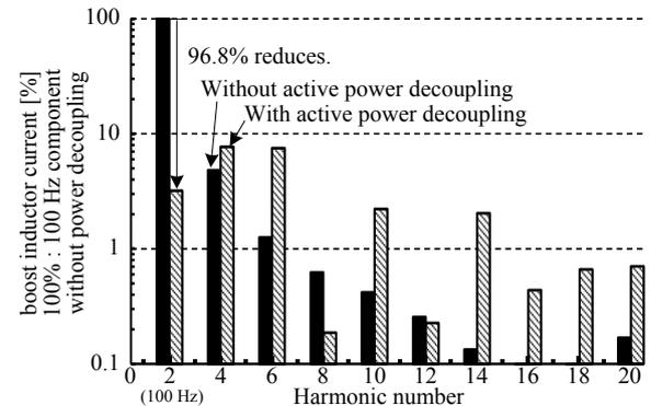
Fig. 5. Harmonics components on the boost inductor current.
