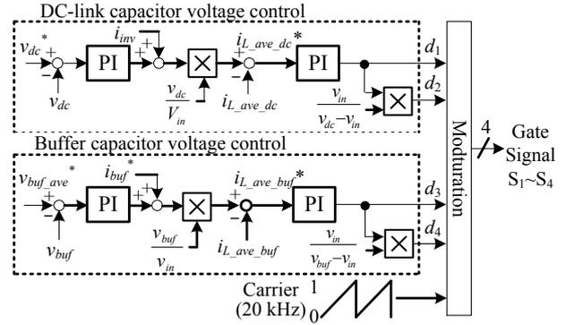
Fig. 3. Control block for DC link voltage and buffer voltage.
