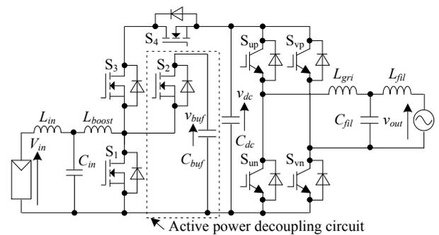
Fig. 1. Active power decoupling circuit operated in DCM.
