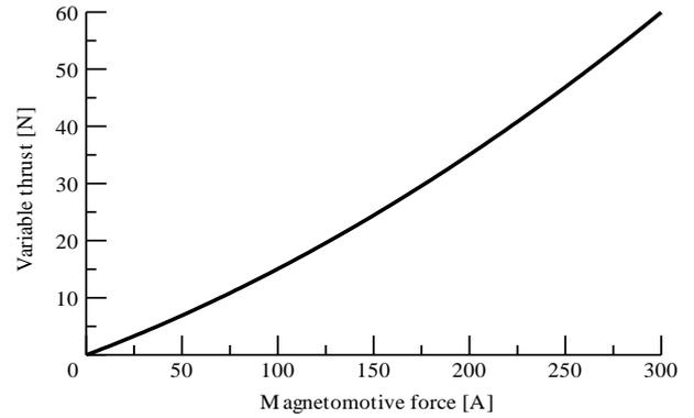
Fig. 5. Analysis result of the variable thrust. The variable thrust is 57.5 N (11.7%) at  $F = 290$  A.
