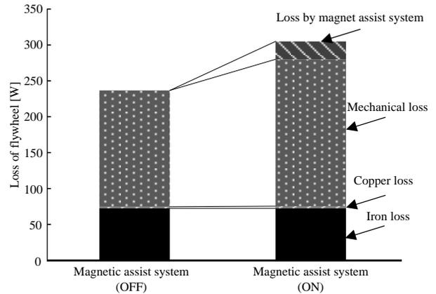
Fig. 8. Analysis result of the loss of flywheel when the steady rotation speed of the flywheel is 6000 r/min and the pressure of the vacuum case is 3.10 Pa. The mechanical loss is increased by 26.2 % by the magnetic assist system.
