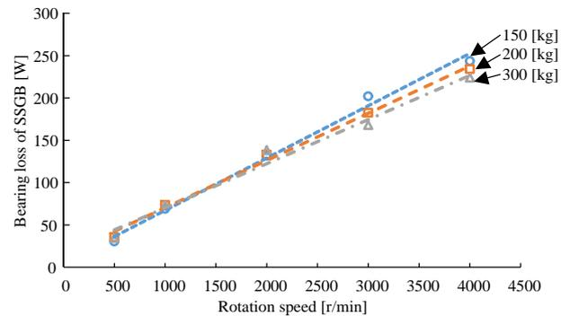
Fig. 9. Measurement result of the bearing loss of the SSGB.
