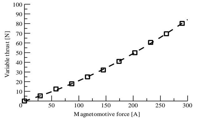
Fig. 6. Measurement result of the variable thrust. The variable thrust is 80.2 N (16.4%) at  $F = 290$  A.
