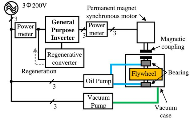
Fig. 1. Block diagram of FESS including measurement system and auxiliary devices.
