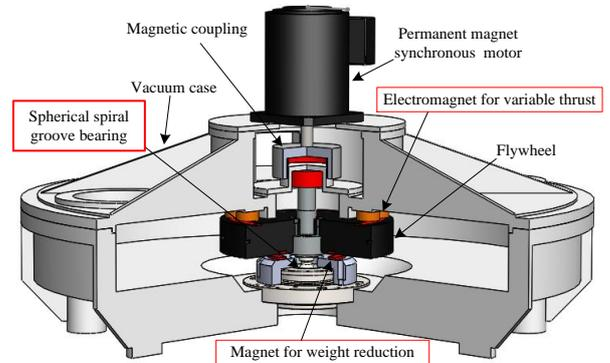
Fig. 2. Configuration of proposed FESS that comprises PMSM, SSGB, and proposed magnetic assist system.
