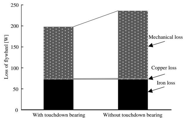
Fig. 7. Analysis result of the loss of flywheel when the steady rotation speed of the flywheel is 6000 r/min and the pressure of the vacuum case is 3.10 Pa. The mechanical loss is increased by 30.4 % without the touchdown bearing.
