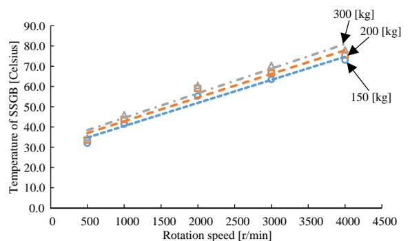
Fig. 10. Measurement result of the temperature characteristic of the SSGB.
