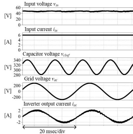
Fig. 14 Simulation result with the proposed converter. The input voltage become constant by active power decoupling.
