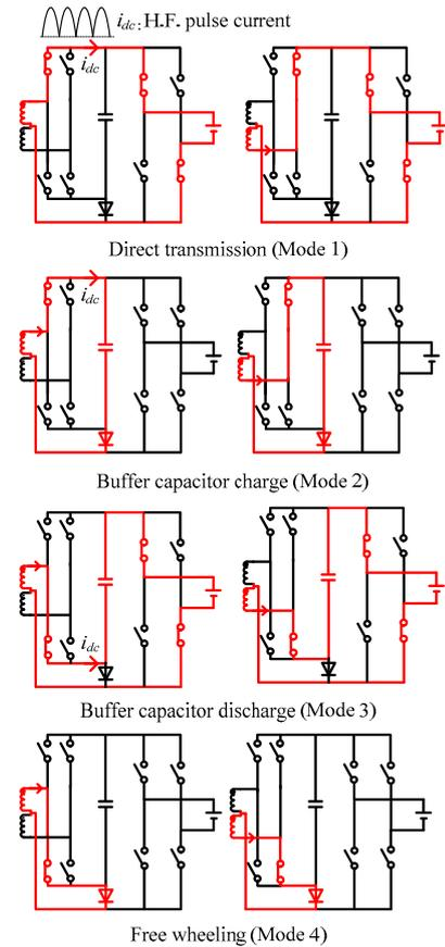
Fig.3 Operation mode of active buffer circuit and CSI. The buffer capacitor is charged and discharged by mode 2 and mode 3. Each mode is switched at the zero current point of the high frequency pulse current.
