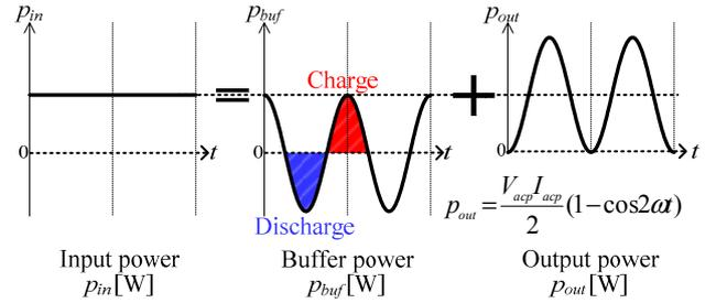
Fig. 2 Compensation principle of the single-phase power pulsation. Small buffer capacitor  $C_{buf}$  eliminates the second-order harmonics on  $P_{in}$ .
