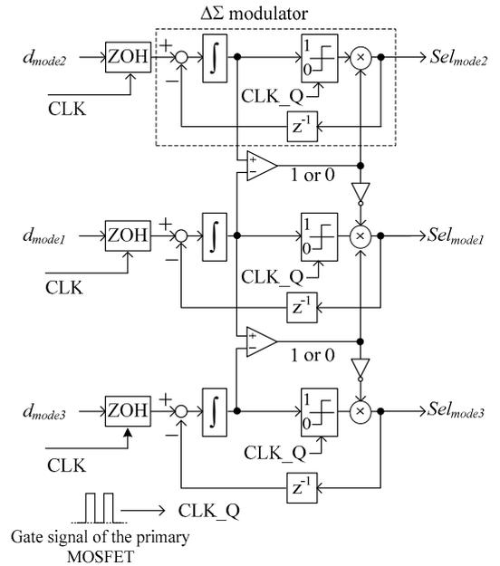
Fig. 5 Modulation block diagram of delta-sigma based pulse density modulation.
