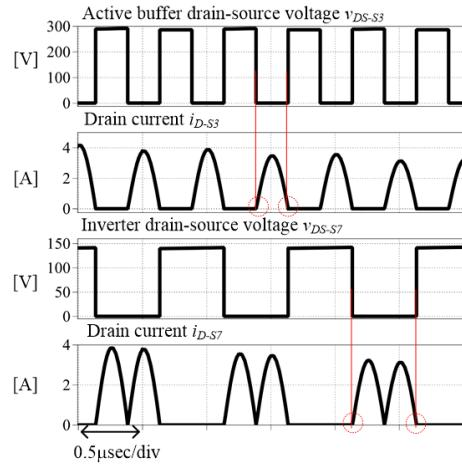
Fig. 15 Each switching waveforms applying the ZCS. The proposed converter can achieve the ZCS including the isolated resonance DC/DC converter.
