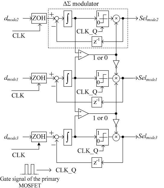
Fig. 5 Modulation block diagram of delta-sigma based pulse density modulation.
