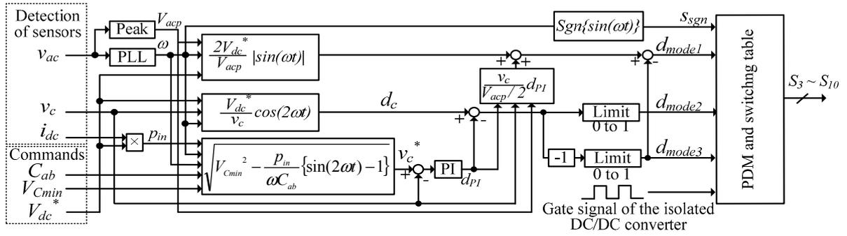
Fig. 4 Control block diagram of active power decoupling circuit and CSI. In order to achieve ZCS, the delta-sigma-based pulse density modulation is applied.
