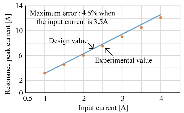
Fig. 12 Comparison between design value and experimental result. The experimental result agrees with the design value.
