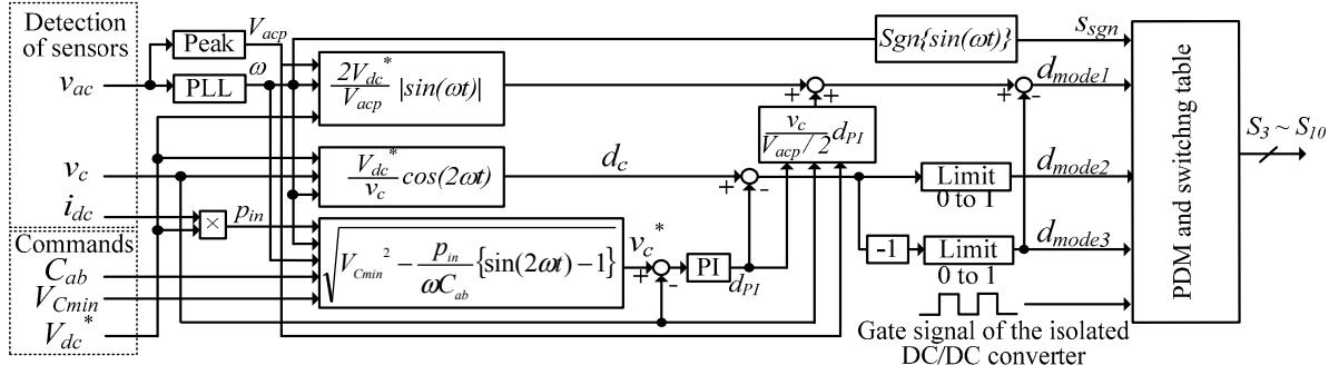
Fig. 4 Control block diagram of active power decoupling circuit and CSI.
