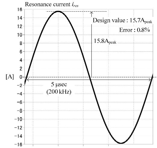
Fig. 8 Simulation result of resonance current. The error between the design and the simulation value is less than 1%.
