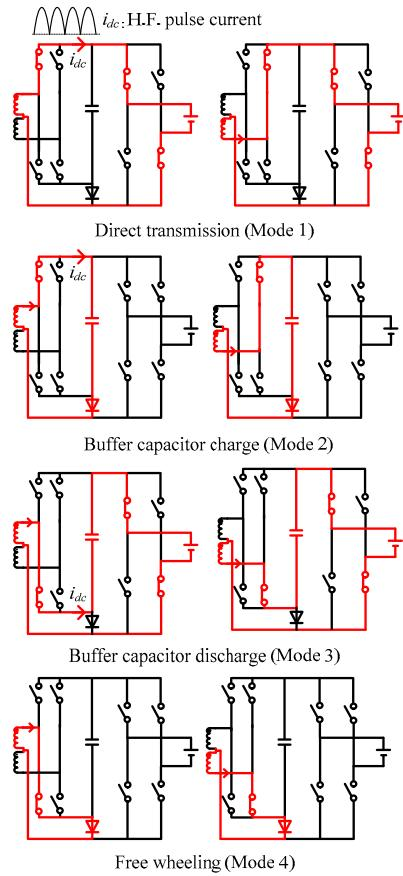
Fig. 3 Operation mode of active buffer circuit and CSI. The buffer capacitor is charged and discharged by mode 2 and mode 3. Each mode is switched at the zero current point of the high frequency pulse current.
