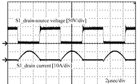
Fig. 11 Experimental result with ZCS of isolated resonance DC/DC converter.
