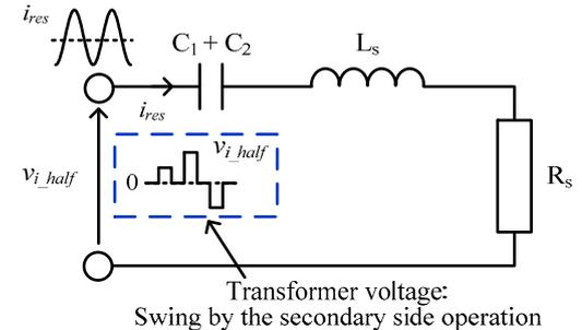
(b) Series resonance model of proposed circuit.
