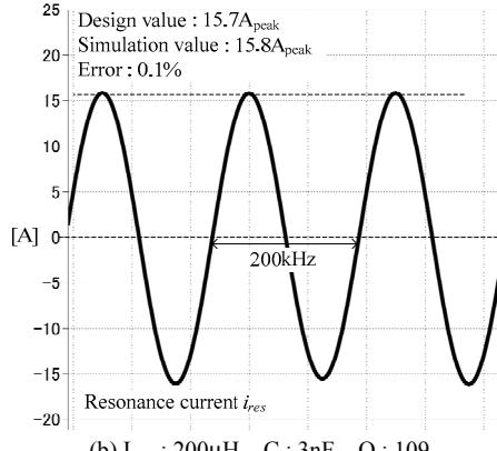
Fig. 10 Resonance current when Q value is changed. When the condition of the low Q value is employed, the error between the design value and the simulation value becomes large.
