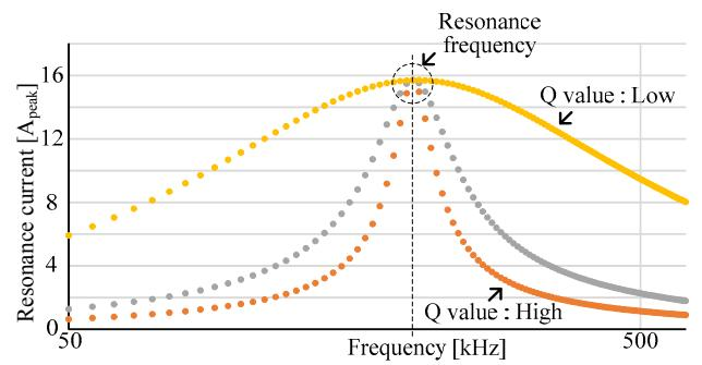
Fig. 7 Characteristics of series resonance current. When the equivalent AC resistance is same, the resonance current peak become maximum at the resonance frequency.
