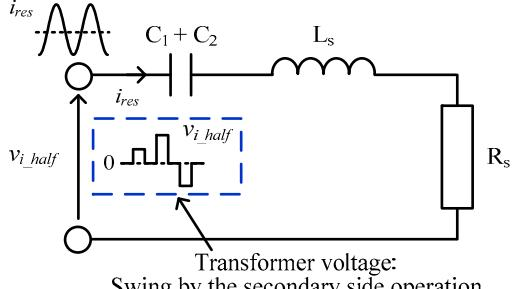
(b) Series resonance model of proposed circuit.
