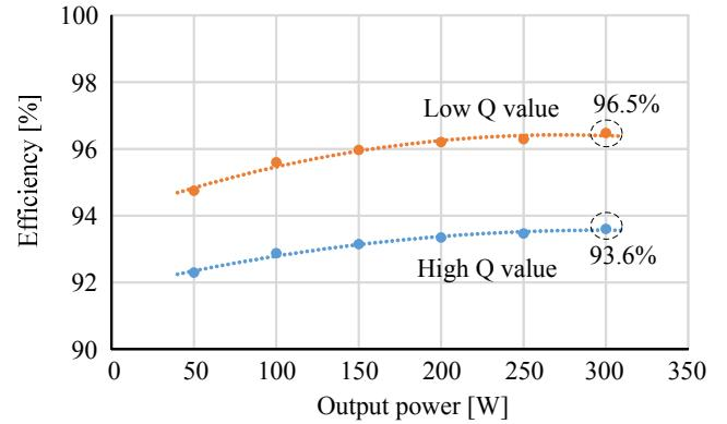
Fig. 13 Efficiency characteristics with isolated DC/DC converter when Q value is changed. In the high Q condition, the efficiency is reduced to 93.6%. This is because the transformer loss is large.
