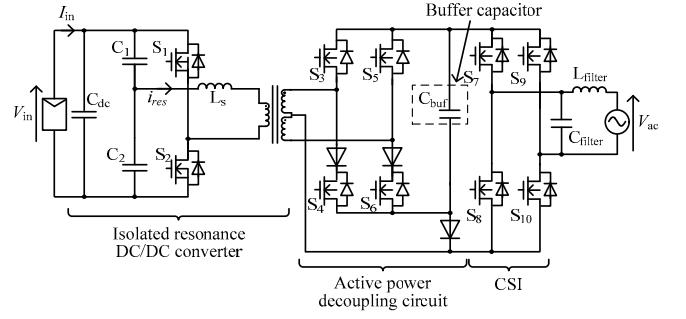
Fig. 1. Proposed DC to single-phase AC grid connected converter which is not required large energy buffer. The proposed converter achieves ZCS on each MOSFETs.
