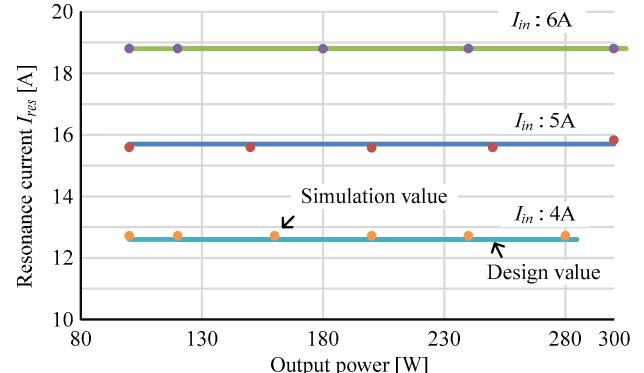
Fig. 9 Comparison between resonance current and design value when output power and input current is changed.
