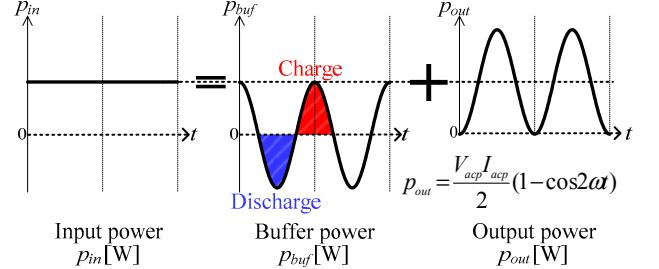
Fig. 2 Compensation principle of the single-phase power pulsation. Small buffer capacitor  $C_{buf}$  eliminates the second-order harmonics on  $P_{in}$ .
