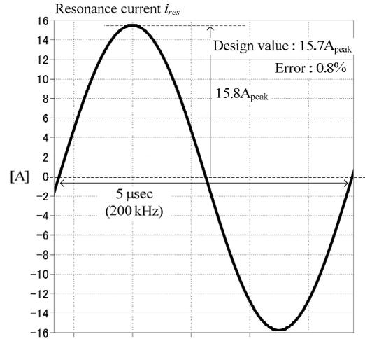
Fig. 8 Simulation result of resonance current. The error between the design and the simulation value is less than 1%.
