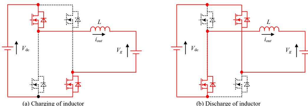
Fig. 2. Equivalent circuit of inverter when grid voltage is positive. The bipolar modulation is applied to reduce common-mode current.
