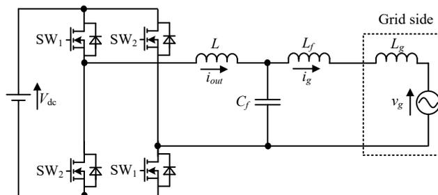
Fig. 1. Single-phase H-bridge grid-tied inverter with LCL filter. A single-phase H-bridge inverter is applied due to its simplicity, which is important for stability analysis and reliability design.
