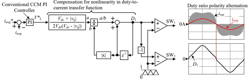
(b) Proposed DCM current control for inverter. In DCM, the switches  $SW_1$  and  $SW_2$  are controlled separately depending on the polarity of the duty ratio, i.e. the polarity of the grid voltage in unity power factor.
