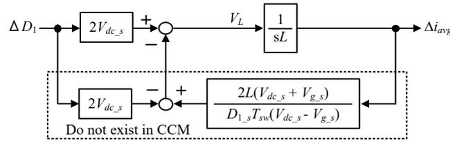
Fig. 5. Linearized circuit model. By estimating the duty ratio at steady states, the DCM nonlinearity can be compensated. Consequently, the controller in DCM can be designed as same as in the CCM operation, which has been researched and analyzed thoroughly.
