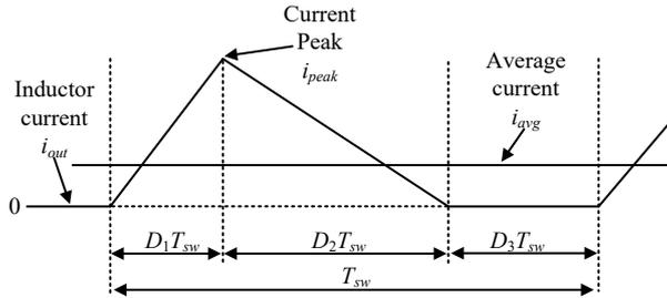
Fig. 3. Inductor current waveform in DCM. The zero-current interval introduces nonlinearities into the DCM operation.
