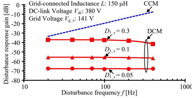
Fig. 9. Disturbance response in CCM and DCM. The DCM nonlinearity in the disturbance-to-current transfer function makes the DCM current more resistant to the disturbance than the CCM current. Therefore, the LCL filter can be further minimized in DCM.
