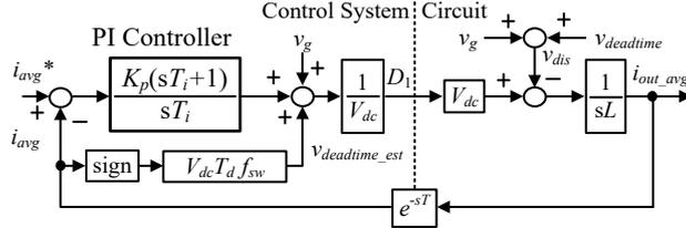
(a) Conventional CCM feedback current control block with typical dead-time error voltage compensation. When the inductance is minimized by reducing the inductance, the inverter becomes more vulnerable to the disturbances, i.e. the increase in the disturbance gain.
