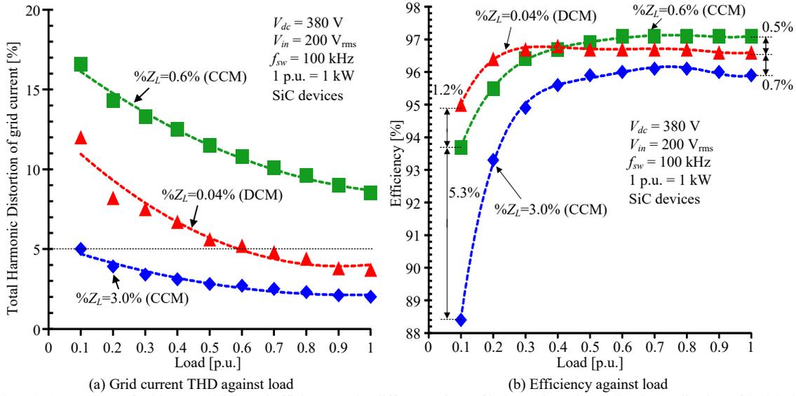
Fig. 14. Comparison of grid current THD and efficiency under different values of inductor impedance. By the application of DCM, the low grid current THD and the efficiency improvement can be achieved.
