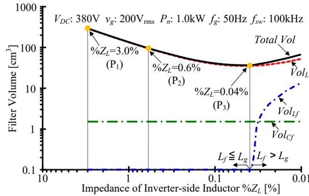
Fig. 11. Relationship between filter volume and inductor impedance at switching frequency of 100 kHz. The filter volume can be minimized greatly when reducing the impedance of the inverter-side inductor.
