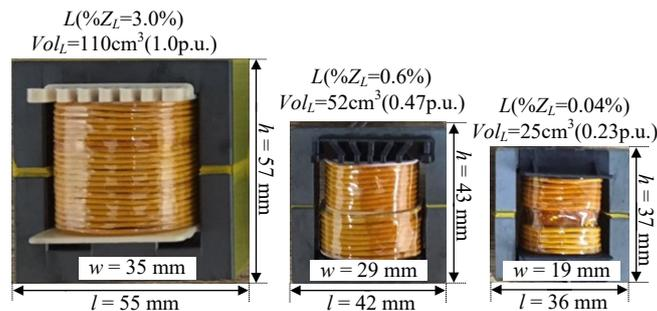
Fig. 12. Prototypes of inverter-side inductors under different condition of inductor impedance. By reducing the impedance of the inverter-side inductor  $\%Z_L$  from 3.0% to 0.04%, the inductor volume is reduced by 77%.
