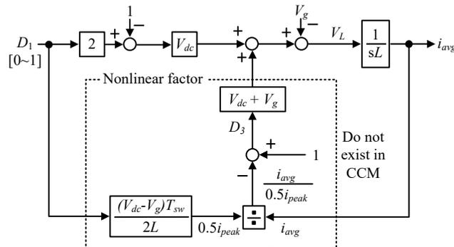
Fig. 4. Circuit model of inverter operated in DCM. In DCM, the current control depends greatly on the current value, i.e. the nonlinearities occurring in the duty-ratio-to-current transfer function and the disturbance-to-current transfer function.
