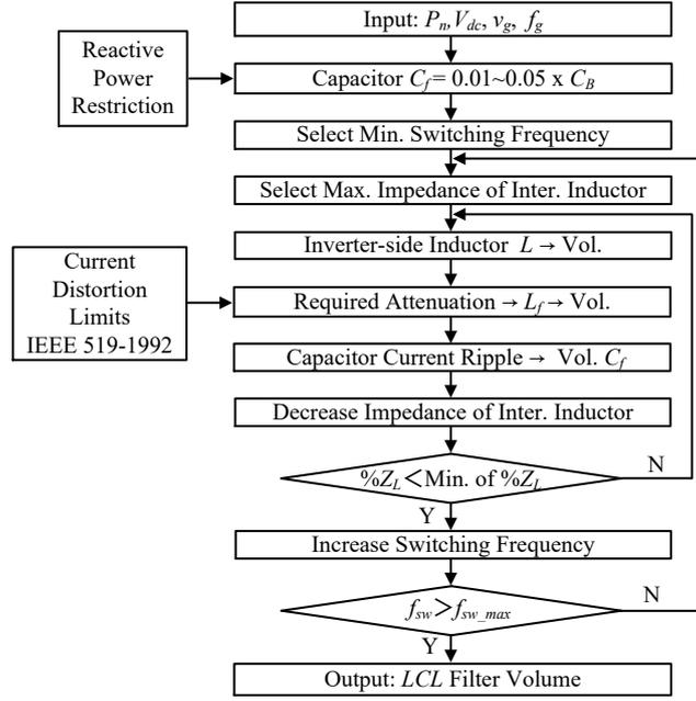
Fig. 10. LCL filter design algorithm. In DCM, the LCL filter can be optimized in aspect of volume or loss because the DCM disturbance gain is much smaller compared to CCM even with a small impedance of the LCL filter.
