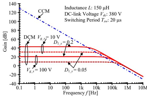
Fig. 6. Bode diagram of duty-ratio-to-current transfer function for CCM and DCM. The zero-current interval in DCM introduces the first nonlinearity into the duty-ratio-to-current transfer function, which greatly worsens the DCM current command response.
