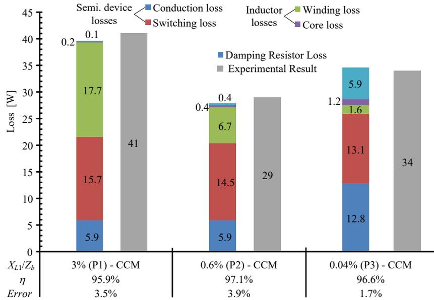
Fig. 15. Volume and loss distribution of at three design points (P1-P3).
