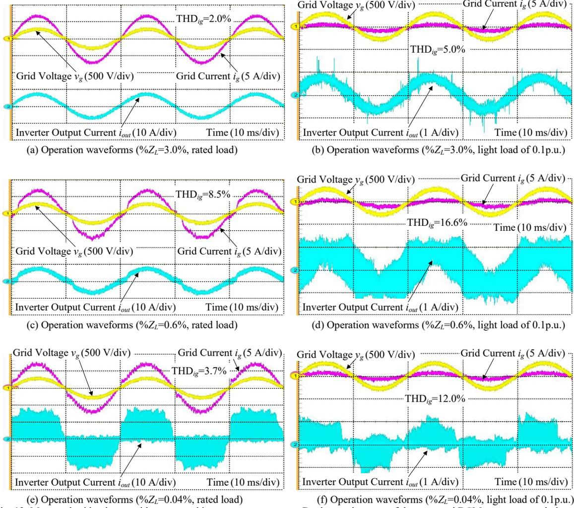
Fig. 13. Measured grid voltage, grid current and inverter output current. By the employment of the proposed DCM current control, the grid current THD below 5% at rated load is achieved even with a small inductor impedance of 0.04%.
