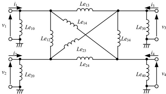
Fig. 5. Equivalent circuit of four-winding transformer. This circuit is extended from the  $\pi$ -type equivalent circuit for two-port network.
