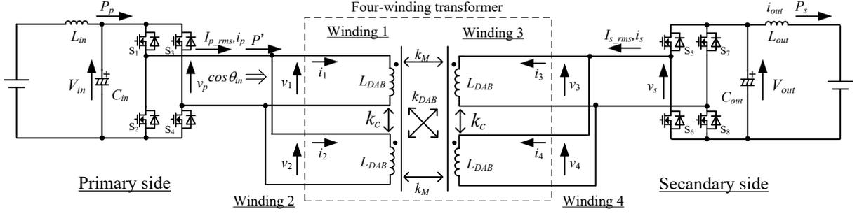
Fig. 4. Circuit configuration of proposed IPT system using four-winding transformer. The cores of the four-winding transformer is shared in each the primary side and the secondary side. The output power  $P_{out}$  is defined as lower value of  $|P_p|$  or  $|P_s|$ .
