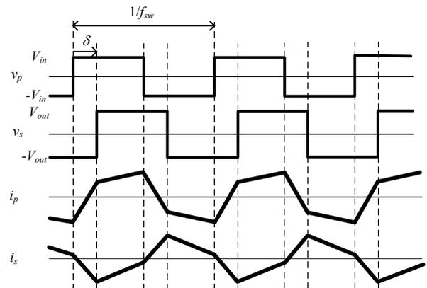
Fig. 3. Voltage and current waveforms of non-resonant IPT system utilized dual active bridge. The inverters are operated as two-level inverter. Polarities of the voltage and directions of the current is defined in Fig. 2.
