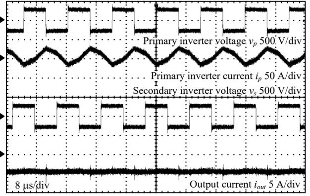
(b) Rated load (1.1 kW) with discharging operation.
