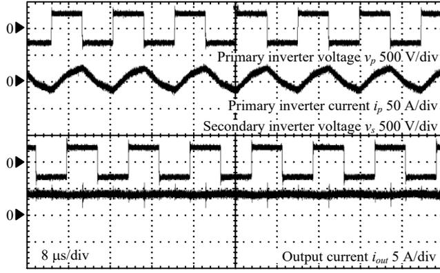
(a) Rated load (1.1 kW) with charging operation.
