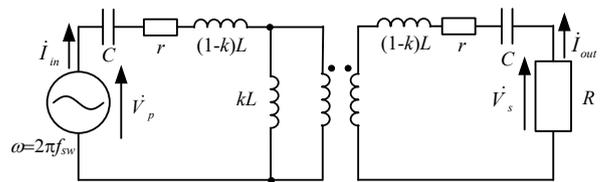
Fig. 1. Equivalent circuit of a S/S resonant IPT system. The self-inductance and the equivalent series resistances  $r$  in each the primary side and secondary side are same value for simplify.
