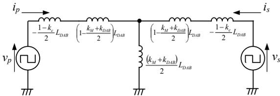
Fig. 6. Equivalent circuit of proposed system. The four-winding transformer is shown as the two-winding transformer. In addition, the two-level full-bridge inverters are shown as the square-wave voltage sources.
