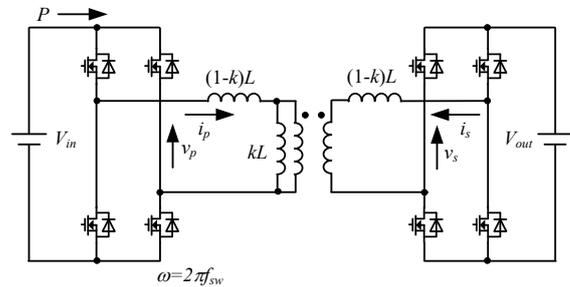
Fig. 2. Non-resonant IPT system applied dual active bridge.
