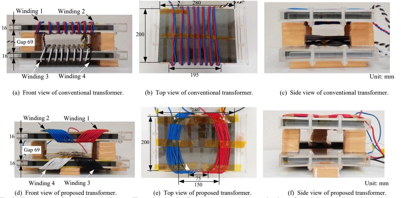
Fig. 9. Two prototype four-winding transformers. The outline drawing from (a) to (c) are the conventional transformer whose windings of the primary or secondary side are close to each other. The outline drawing from (d) to (f) are the proposed transformer whose windings of the primary or secondary side are separated to introduce the proposed method.
