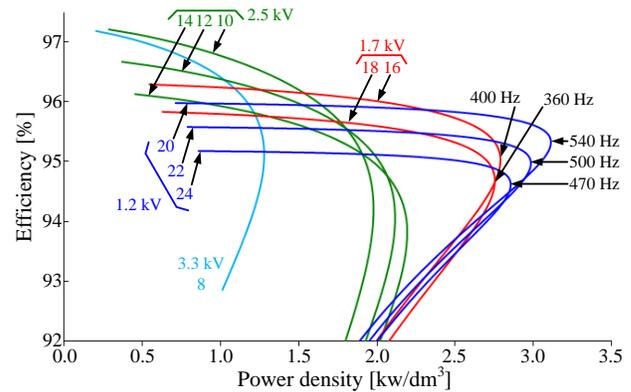
Fig. 29. Expanded Pareto front curve at an MMC output voltage of 1200 V without a 3.3 kV SiC. The converter applied to a 1.7 or 1.2 kV IGBT produces a higher power density except for the 3.3 kV SiC. Moreover, both 1.7 and 1.2 kV IGBT produce the highest power density when the lowest number of cells is employed.
