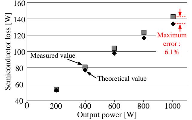
Fig. 24. Comparison of theoretical and measured semiconductor losses. The maximum error is 6.1%. This error is attributed to losses from the equivalent series resistance (ESR) of the capacitor and the wiring loss, which are not considered in the calculations.
