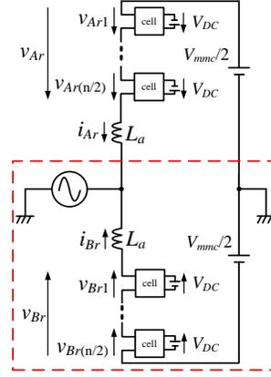
Fig. 11. Equivalent circuit model of the single phase circuit in the MMC. The cell capacitor is replaced by an ideal voltage source.
