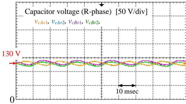
Fig. 17. Waveforms for the capacitor voltage in the R-phase leg. The proposed system maintains the capacitor voltage of each H-bridge cell to the voltage command of 130 V. In addition, the maximum voltage error between the capacitor voltage command and the measured voltage is 2% or less.
