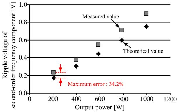
Fig. 20. Comparison of theoretical and measured values for the second-order frequency component in the ripple voltage. The maximum error between the theoretical value and the measured value is 34.2%. The cause of the large error is the mismatch of the input active power and the output power due to the semiconductor loss and the inductor loss.
