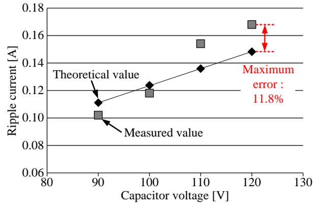
Fig. 23. Comparison of the theoretical and measured ripple currents in the arm inductor against capacitor voltage. The maximum error is 11.8%. This error results because the inductance decreases due to the decrease of the permeability as the core temperature is raised.
