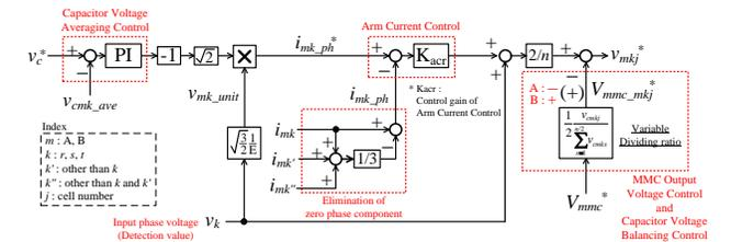
Fig. 3. Control block diagram for each arm in H-bridge cell type MMC. Note that  $m$  is the index of the arm group A or B,  $k'$  or  $k''$  is the index of the phase such as  $r$ ,  $s$  and  $t$ , and  $j$  is the index of the cell number.
