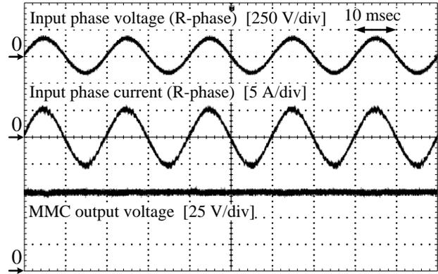
Fig. 15. Waveforms for input voltage, input current and output voltage. The unity power factor is obtained in the input stage. The THD of the input current is 3.2% when the %Z of the inductor is 6.1%.
