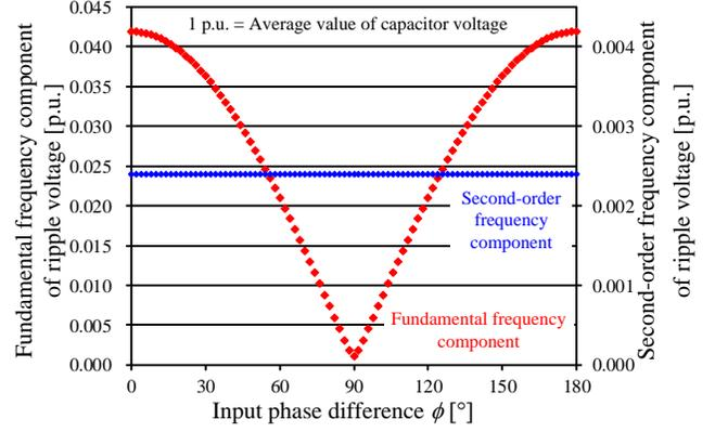
Fig. 5. Relationship between input phase difference  $\phi$  and ripple voltage. The fundamental frequency component is maximum when  $\phi$  is 0 or  $\pi$ .
