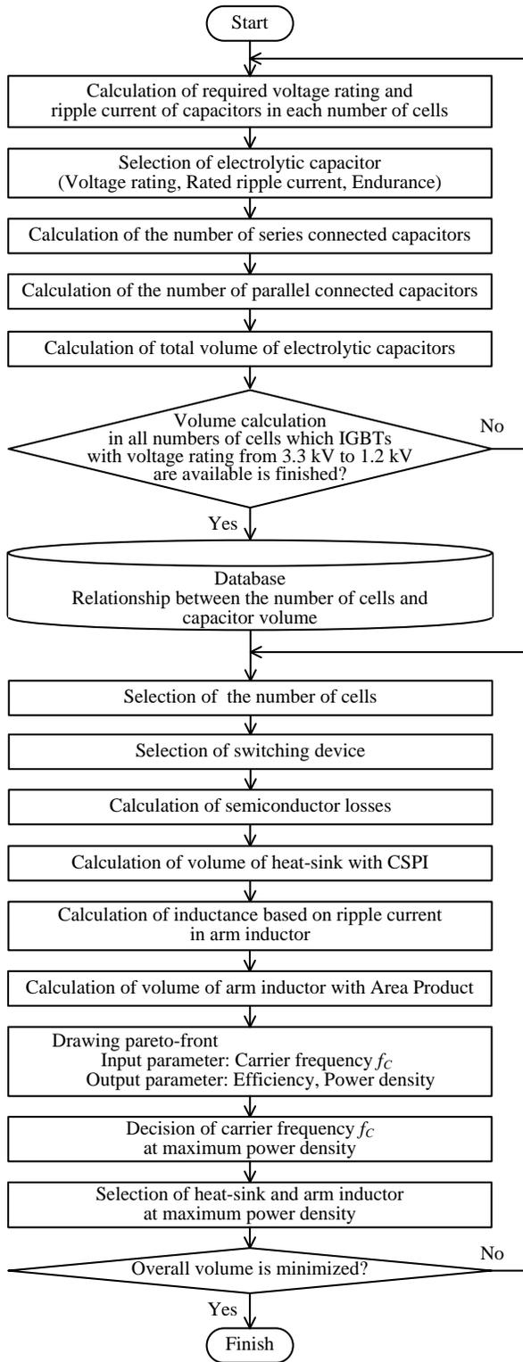
Fig. 4. Design flowchart for a step-down rectifier with MMC.
