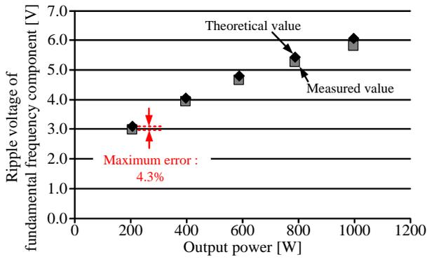
Fig. 19. Comparison of theoretical values and measured data for the fundamental frequency component of the ripple voltage. The maximum error between the theoretical and measured values is 4.3%.
