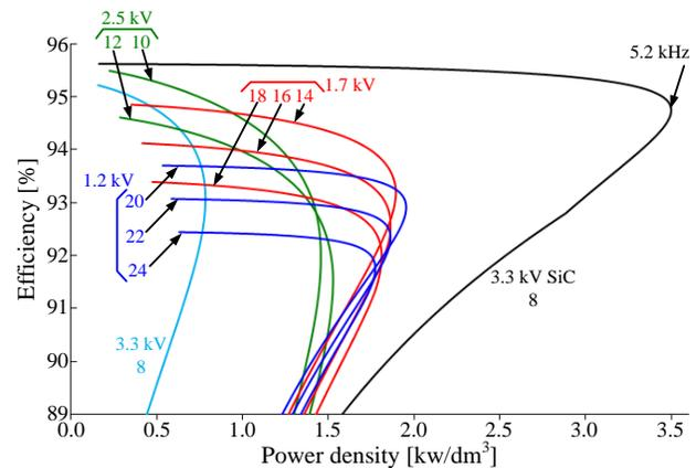
Fig. 27. Pareto front curve for an MMC output voltage of 800 V. The power density of the converter applied to the 3.3 kV SiC is approximately two times higher compared to the converter applied to other switching devices.
