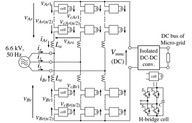
Fig. 2. Circuit configuration of front-end converter with H-bridge cell type MMC and isolated DC-DC converter.
