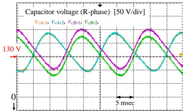
Fig. 18. Waveforms for the ripple voltages of all capacitors that are connected to the R-phase leg. In principle, each capacitor in the MMC has a low frequency ripple voltage because the frequency of the ripple voltage is based on the frequency of the input voltage source.
