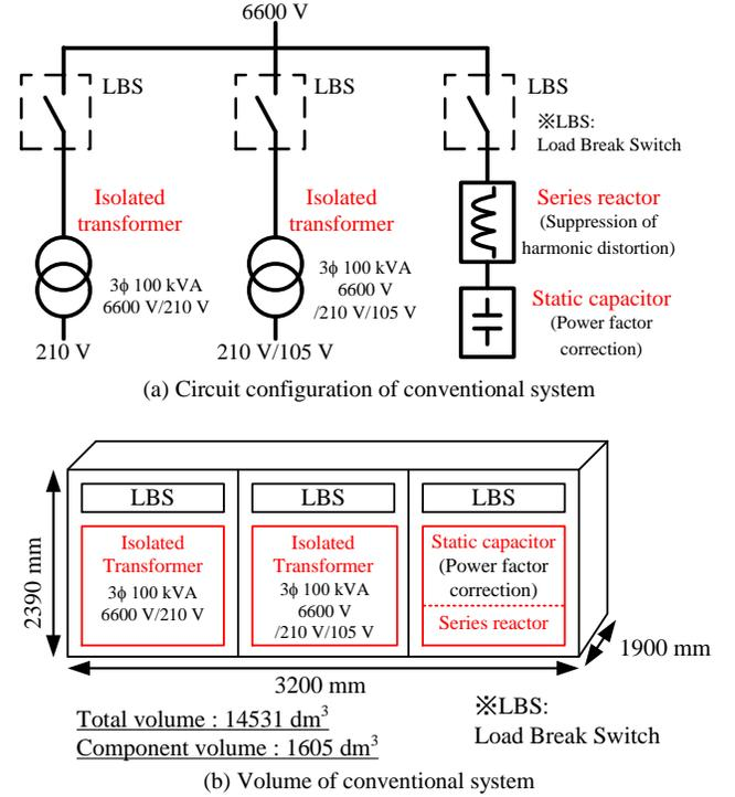
Fig. 1. Conventional power system of 200 kVA connected to utility grid of 6.6 kV. The conventional power system is constructed of several bulky transformers, a high capacity static capacitor and a series reactor.
