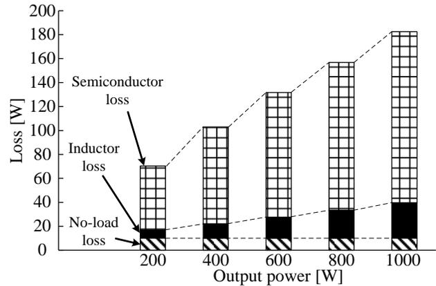
Fig. 25. Breakdown of losses in the MMC. The no-load loss is constant despite varying the output power. In contrast, the semiconductor and inductor losses increase with increases in the output power because the arm current is elevated.
