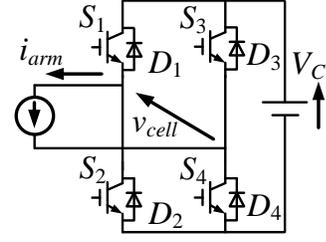
Fig. 8. Circuit model of the H-bridge cell for loss analysis.
