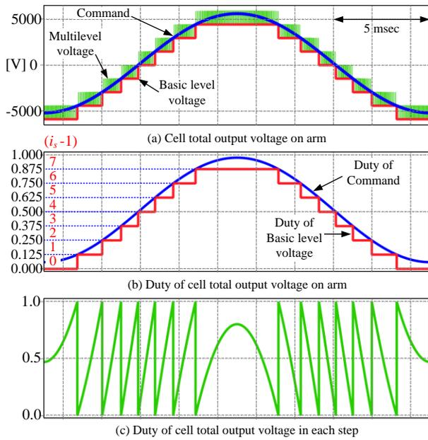
Fig. 13. Command for the cell total output voltage, the multilevel waveform for the total output voltage and the basic level voltage. Each duty of the cell total output voltage and basic level are also shown, as are the duty of the cell total output voltage in each step,  $d_{mbl}$ .
