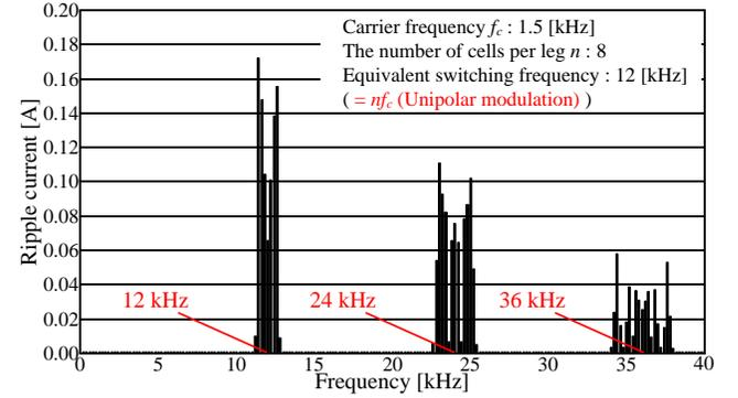
Fig. 12. Frequency analysis of the ripple current. The frequency of the ripple current on each arm inductor is determined by the equivalent switching frequency  $f_{ic\_eq} = nf_c$ .
