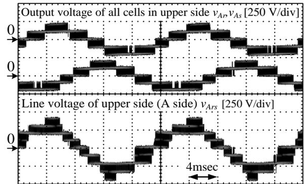
Fig. 16. Waveforms for arm voltage which is the summation of output voltage of all cells in each arm and waveforms of line voltage between R-phase and S-phase in upper side. The arm voltage is five levels and the line voltage is nine levels.
