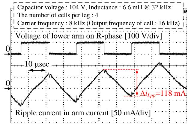
Fig. 22. Waveforms for lower arm voltage in R-phase and arm current. The expanded waveforms focus on the output voltage of which the duty in each step of the cell total output voltage,  $d_{mlvs}$ , is 0.5. The error between the theoretical value and the measured value is 4.9%.
