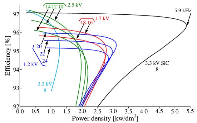
Fig. 28. Pareto front curve at an MMC output voltage of 1200 V. All switching devices achieve higher power density and higher efficiency compared to the evaluation result with the MMC output voltage of 800 V.
