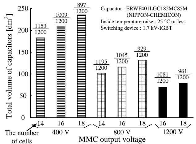
Fig. 26. Change in the capacitor volume against the MMC output voltage. The values under the graph indicate the number of cells for which a 1.7 kV IGBT is available. At the same output voltage, the capacitor volume is small when the voltage rating ratio is high.
