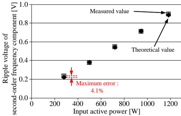
Fig. 21. Comparison of the theoretical and measured values of the second-order frequency component based on input active power. The maximum error between the theoretical and measured values is 4.1%.
