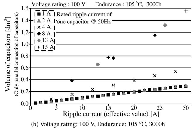
Fig. 6. Relationship between ripple current and capacitor volume. The parallel connection of capacitors with small rated ripple currents rather than only one capacitor with a large rated ripple current results in size reduction.
