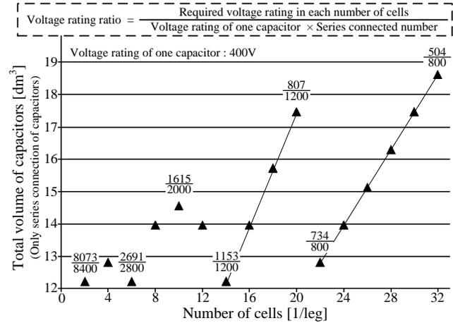
Fig. 7. Relationship between the number of cells and the capacitor volume. The capacitor volume becomes small when the voltage rating ratio is close to 1.0.
