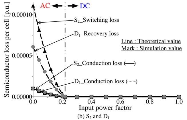
Fig. 10. Comparison result of theoretical formula of semiconductor loss and simulation.
