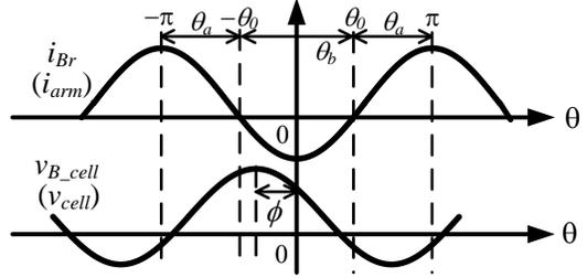
Fig. 9. Relationship between the cell output voltage and the arm current in the lower side of the MMC.
