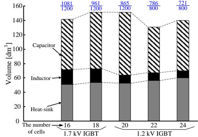
Fig. 30. Breakdown of the overall volume for an MMC output voltage of 1200 V and a 1.7 or 1.2 kV IGBT. The change in the capacitor volume is particularly large. From the above results, the first step in the design of the MMC should focus on the number of cells for which the capacitor volume is small based on the voltage rating ratio.
