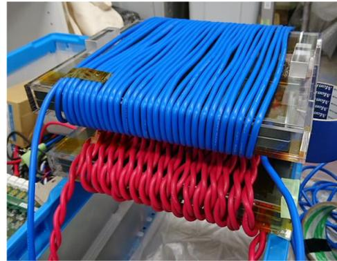
Fig. 5. Transmission coils which is used core with PC40 manufactured by TDK. Upper side is transmitter coil, lower side is receiver coil. Coil size is  $W237 \times H210 \times D20$  mm. Transmission distance is 50 mm.
