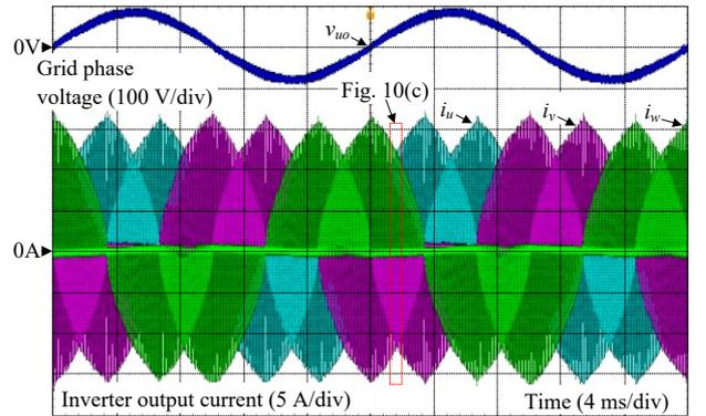
(b) Grid phase voltage of u phase, and three-phase inverter output currents
