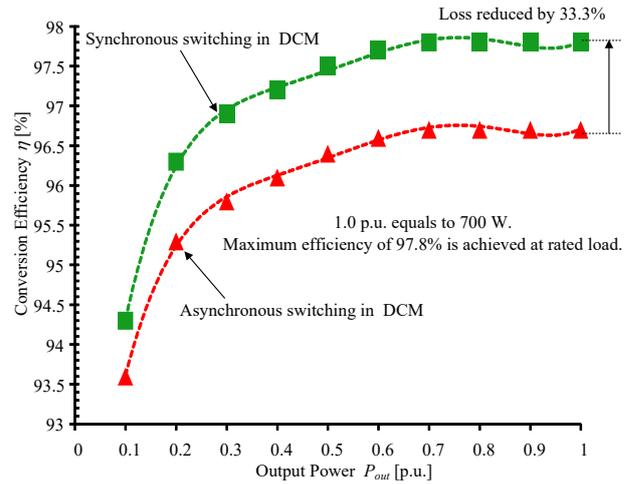
Fig. 14. Efficiency comparison between asynchronous switching and synchronous switching in DCM. The application of the DCM synchronous switching reduces the conversion loss by 33% compared to the DCM asynchronous switching at rated load.
