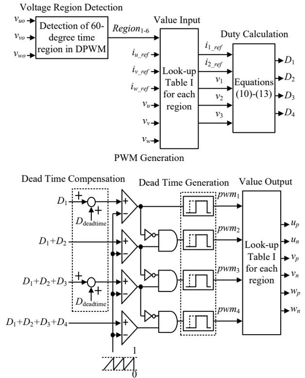
Fig. 4. Control system of the three-phase grid-tied inverter operating completely in DCM. The dead-time-induced error voltage is compensated simply when the inverter is intentionally operated in DCM because the zero-current interval is controlled.
