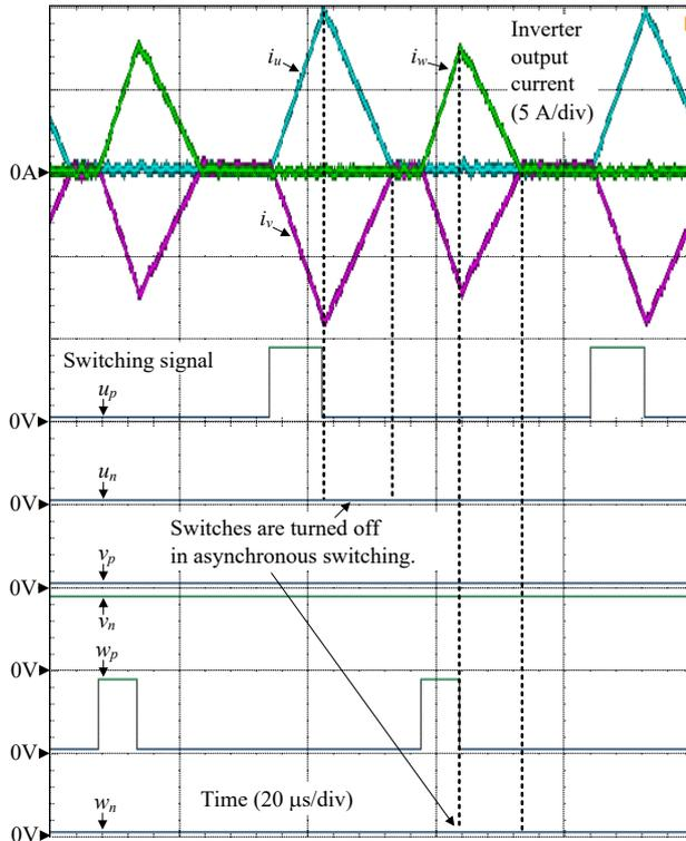
(a) Asynchronous switching in DCM
