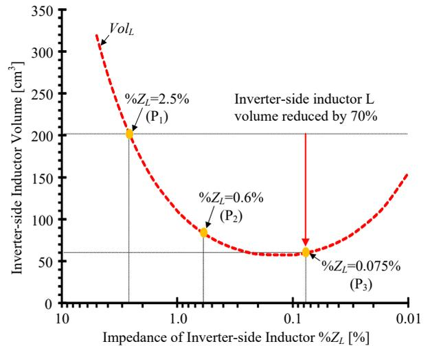
Fig. 5. Relationship between filter volume and inductor impedance at switching frequency of 40 kHz. The inductor volume can be minimized greatly when reducing the inductor impedance.
