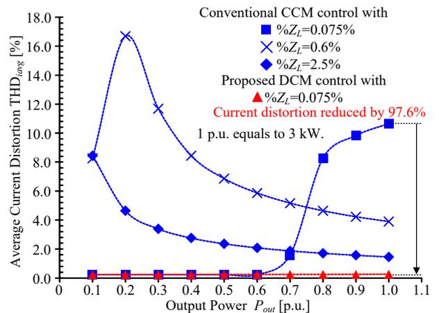
Fig. 8. Current THD characteristics of conventional CCM current control and proposed DCM current control with three different inductor designs. With the proposed DCM current control, the current THD is maintained below 5% over entire load range from 0.1 p.u. to 1.0 p.u..
