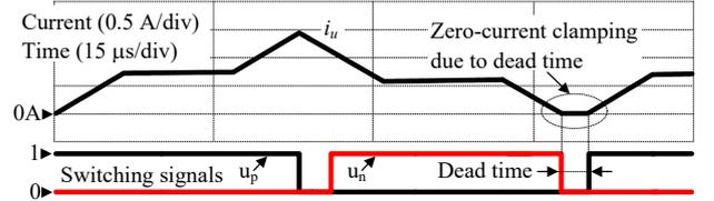
(b) Zero-current clamping effect due to dead-time
