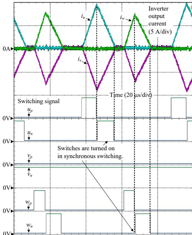
(b) Synchronous switching in DCM
