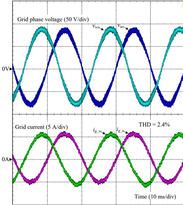
(a) Grid phase voltages and grid currents of u phase and w phase at normal operation
