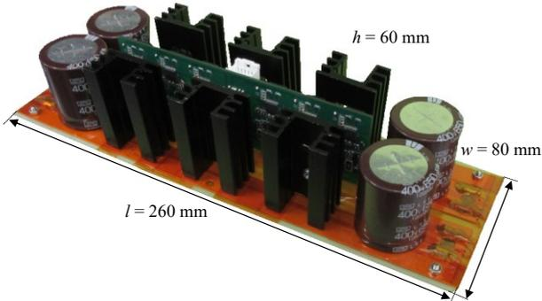
Fig. 9. Prototype of miniature three-phase grid-tied inverter.
