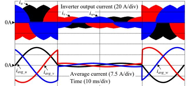
Fig. 7. Load step response between load of 0.1 p.u. and load of 1.0 p.u.. The stable inverter operation is confirmed even at load step change.
