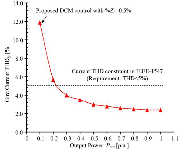
Fig. 12. Current THD characteristics of proposed DCM current control. The current THD is maintained below 5% over load range from 0.3 p.u. to 1.0 p.u., which satisfies the current THD constraint in IEEE-1547, even when the inductance impedance is reduced to 0.5% of the inverter impedance.
