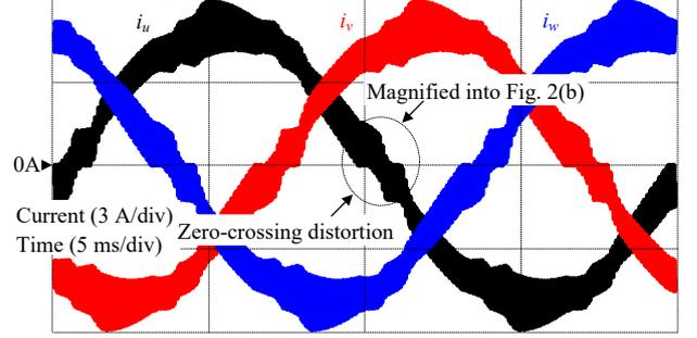
(a) Zero-crossing distortions in inverter output currents
