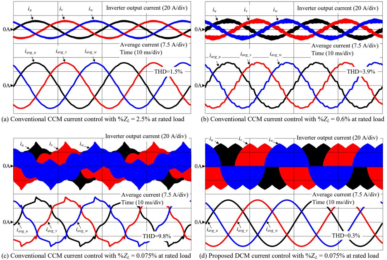
Fig. 6. Inverter output currents and average currents of conventional CCM current control and proposed DCM current control at rated load. The current THD of the conventional CCM current control increases with the reduction of the grid filter impedance, whereas the current THD of the proposed current control is still low.
