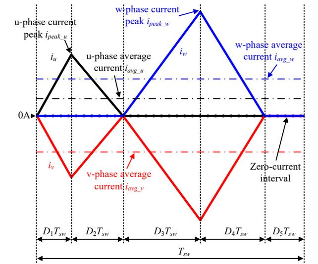
(b) Inverter output current waveform in one switching period during 0°-60° region
