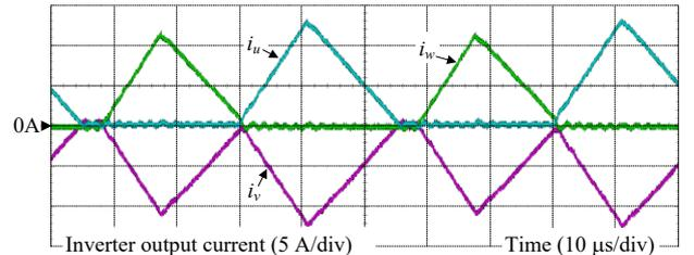
(c) Zoom-in three-phase grid current from Fig. 10(b)
