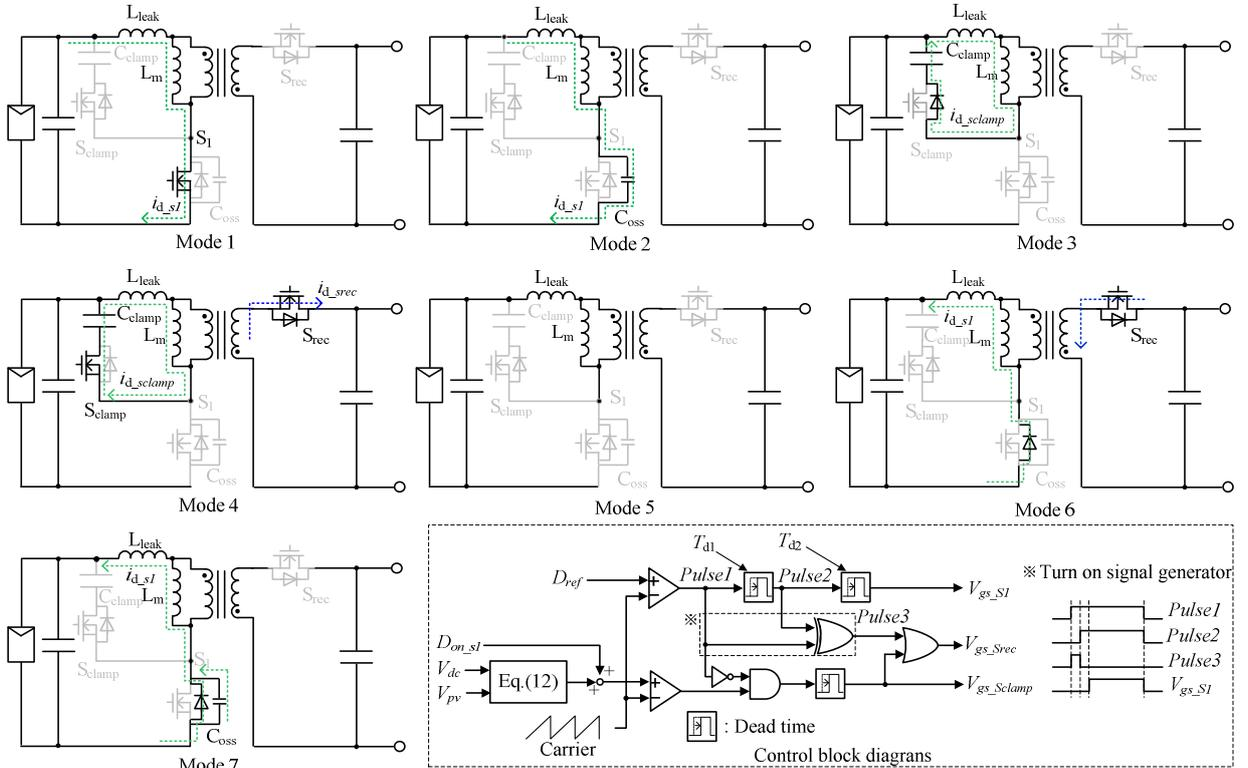
Fig. 7. Operation modes and the control block diagrams of flyback converter. In order to achieve ZVS, mode 6 and 7 which discharge the parasitic capacitor are proposed.
