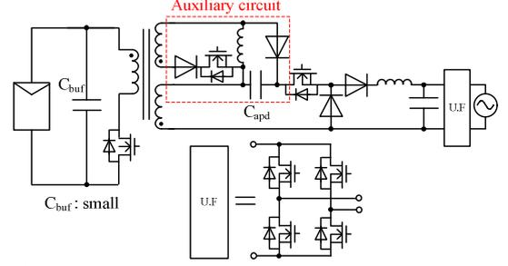
Fig 1. Conventional flyback micro inverter with active power decoupling circuit. It can reduce the capacitance of  $C_{buf}$ . However, auxiliary circuit is necessary.
