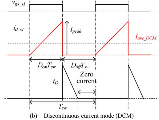
Fig.4. Fundamental waveforms without active clamp circuit. In DCM, power decoupling can achieve under constant duty reference and switching frequency condition.
