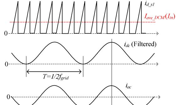
Fig.5. Current waveforms of PV input current  $I_{\text{ave}, \text{DCM}}$ , DC link current  $i_{dc}$  and inverter output current  $i_{ac}$ . DC link capacitor is charged and discharged due to double-line frequency in order to compensate the differential power during input and output power.
