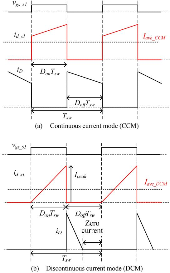
Fig.4. Fundamental waveforms without active clamp circuit. In DCM, power decoupling can achieve under constant duty reference and switching frequency condition.
