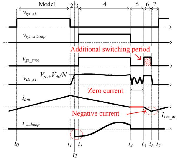
(b) Proposed ZVS method with active clamp circuit. Fig.6. Key waveforms of flyback converter in switching cycle. In order to achieve ZVS, negative current period is necessary before  $S_1$  is turned-on. In addition, zero current period is required for proposed active power decoupling capability.
