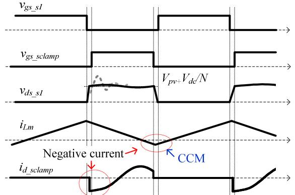
(a) Conventional ZVS method with active clamp circuit. This method, active clamp circuit and main circuit are switched to complementation.
