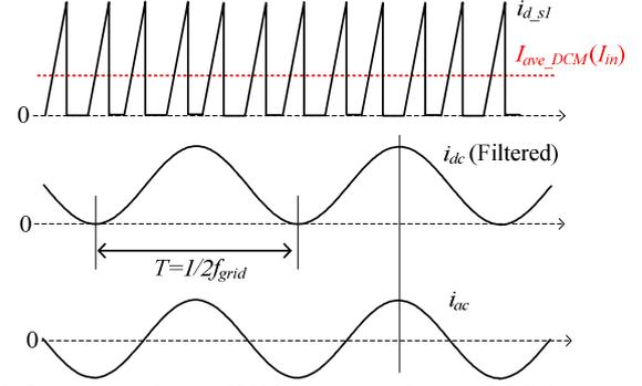
Fig.5. Current waveforms of PV input current  $I_{\text{ave\_DCM}}$ , DC link current  $i_{dc}$  and inverter output current  $i_{ac}$ . DC link capacitor is charged and discharged due to double-line frequency in order to compensate the differential power during input and output power.
