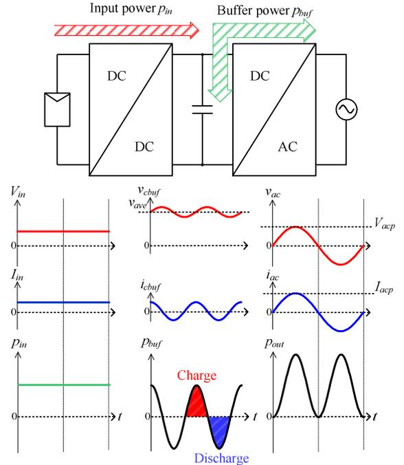
Fig 3. Relationship between input and output power. DC link capacitor receives differential power due to double-line frequency power ripple, and input power becomes constant.
