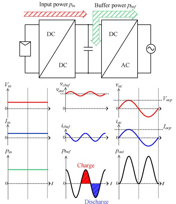
Fig. 3. Relationship between input and output power. DC link capacitor receives differential power due to double-line frequency power grid, and input power becomes constant.
