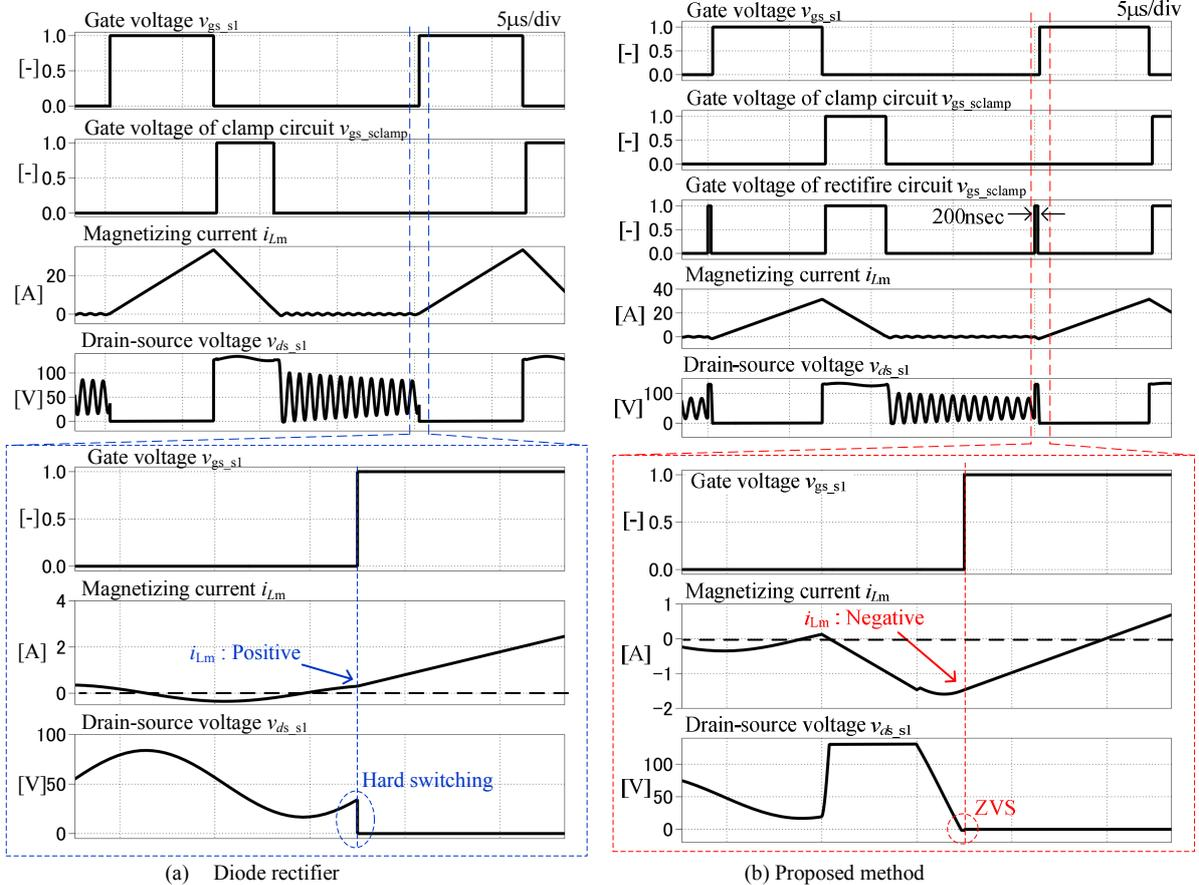
Fig.8. Simulation result with switching waveforms both diode rectifier and proposed method
