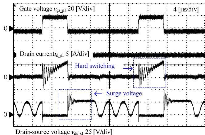
Fig.10. Experimental results with snubber less and diode rectifier condition.
