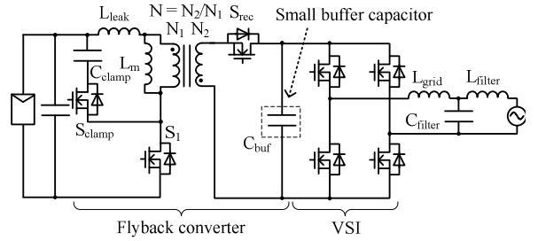
Fig. 2. Circuit configuration of proposed flyback converter. Active clamp circuit suppress turn-off surge voltage. Synchronous rectifier utilizes ZVS operation for  $S_1$ .
