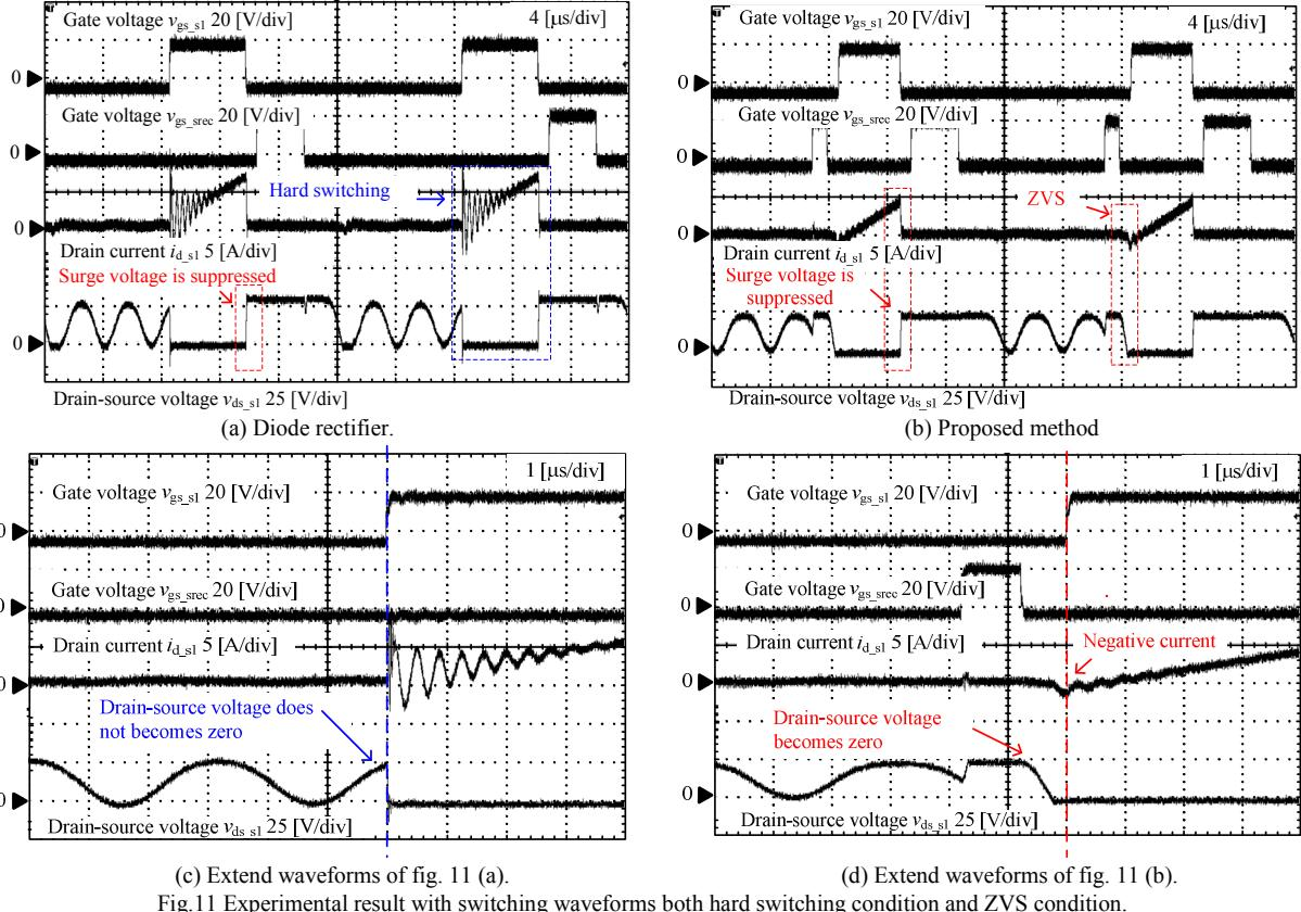
Fig.11 Experimental result with switching waveforms both hard switching condition and ZVS condition.
