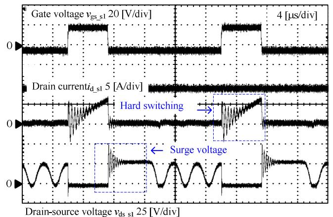
Fig.10. Experimental results with snubber less and diode rectifier condition.
