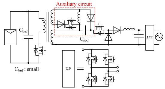
Fig. 1. Conventional flyback micro inverter with active power decoupling circuit. It can reduce the capacitance of  $C_{buf}$ . However, auxiliary circuit is necessary.
