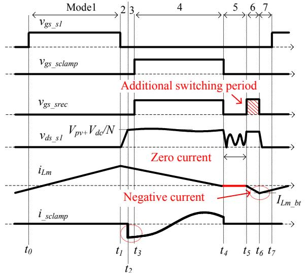
(b) Proposed ZVS method with active clamp circuit.
