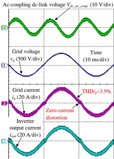
(c) Conventional CCM control,  $\%Z_L=1.8\%$ , light load of 2 kW
