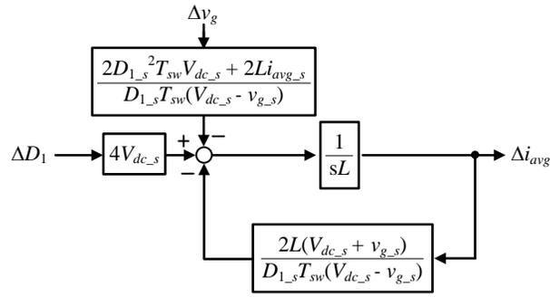
Fig. 5. Linearized circuit model of inverter operating in DCM. The current control of DCM obtains the same dynamic as in CCM by compensating the DCM nonlinearity at the output of the controller.
