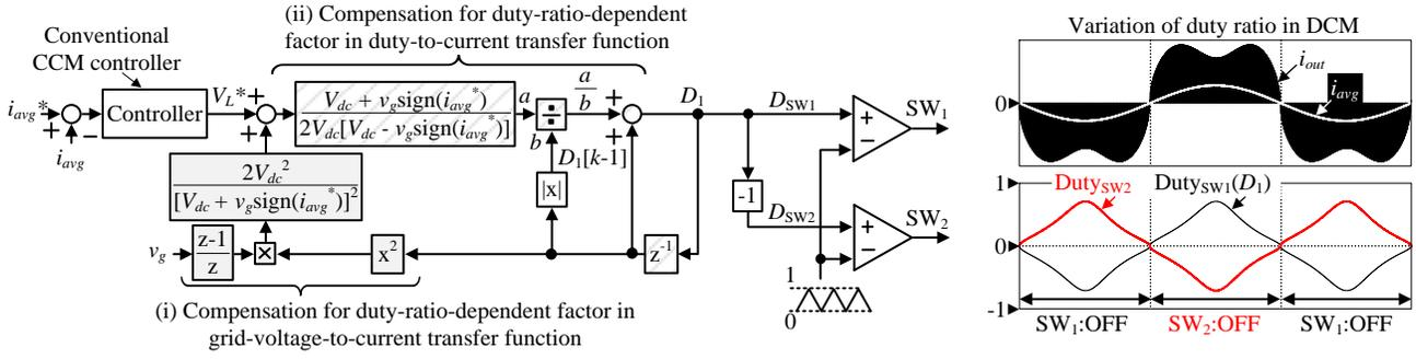
Fig. 10. Proposed DCM current control system for single-phase grid-tied inverter and variation of duty ratio in DCM. The polarity of  $D_1$  is used to determine if  $D_1$  should be applied to  $SW_1$  or  $SW_2$  in order to avoid the interruption of the continuous change of  $D_1$ .
