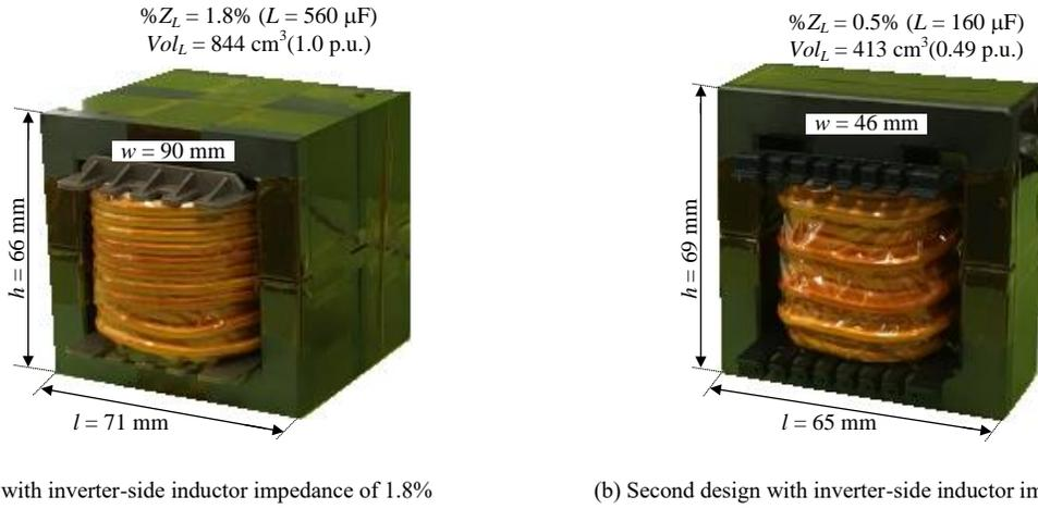
(a) First design with inverter-side inductor impedance of 1.8%
