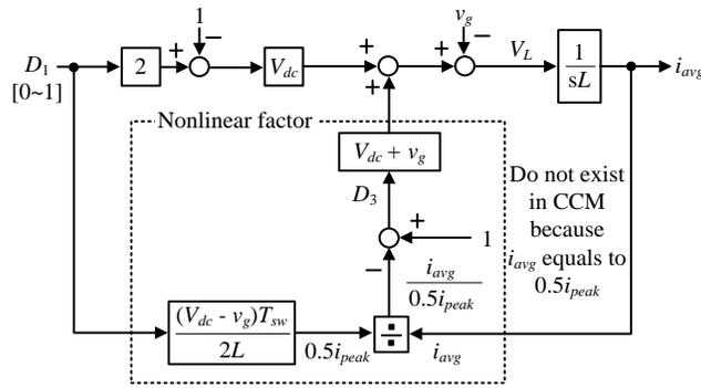
Fig. 4. Circuit model of inverter operating in DCM. The current control loop gain in DCM depends on the average current, i.e. the nonlinearities occurring in the duty-ratio-to-current transfer function and the grid-voltage-to-current transfer function.
