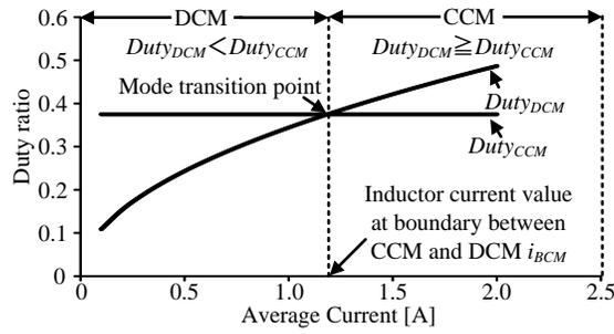
Fig. 11. Relationship among CCM duty, DCM duty and current mode. When the circuit operates in DCM, the DCM duty becomes smaller than the CCM duty and vice versa. The current mode determination is realized independently from the inductor value by using this relationship of the duty ratios.
