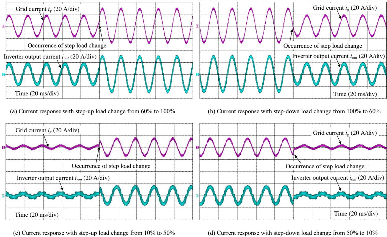
Fig. 19. Proposed CCM/DCM current control operation under step load change with  $\%Z_L$  of 0.5%. The transient waveform has low overshoot and fast convergence when the step load change occurs either in the vicinities of the zero-current crossing, i.e. the DCM interval, or at the current peak, i.e. the CCM interval.
