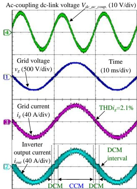
(b) Proposed CCM/DCM control,  $\%Z_L = 0.5\%$ , rated load of 4 kW
