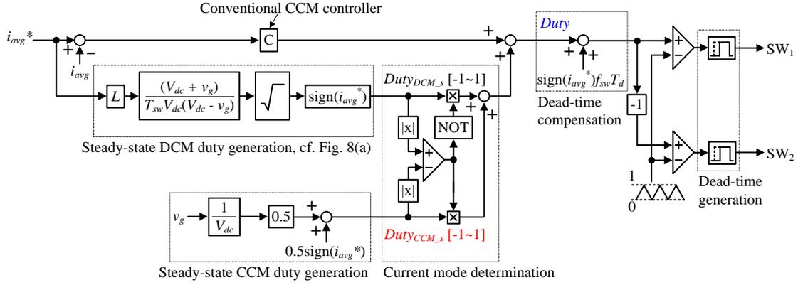
(b) Conventional CCM/DCM current control system, cf. Fig. 10 of [14]
