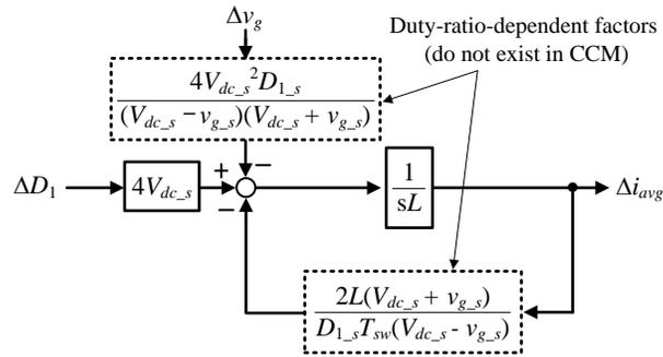
Fig. 6. Simplified and linearized circuit model. The value of the duty ratio  $D_{1_s}$  at steady-state points is required in order to compensate for the duty-ratio-dependent factors occurring when the inverter operates in DCM.
