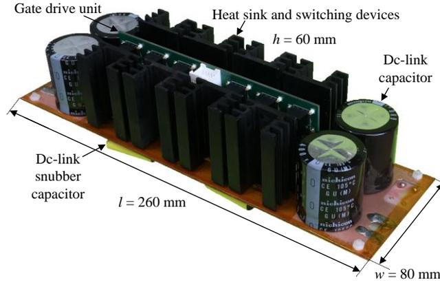
Fig. 13. 4-kW 100-kHz prototype of single-phase grid-tied inverter. SiC switching devices are chosen to operate the inverter at high switching frequency of 100 kHz, whereas two switching devices are connected in parallel to reduce the conduction loss in each device and enable the employment of natural cooling. Meanwhile, four electrolytic capacitors of 680-μF are connected in parallel at the dc link to absorb the single-phase power fluctuation and maintain a low dc-link voltage ripple.
