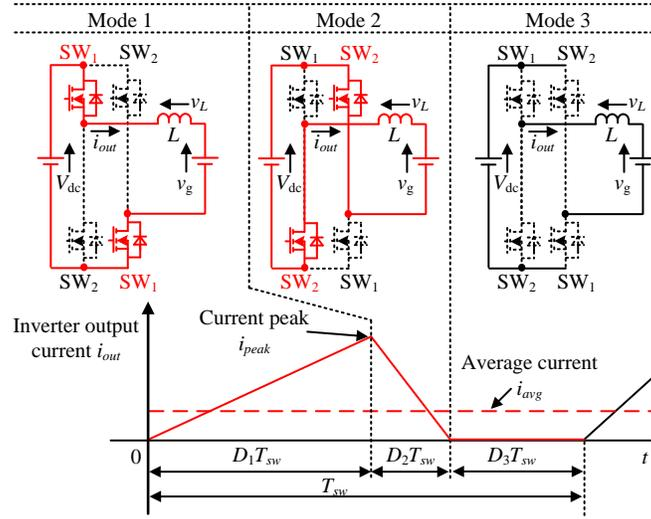
Fig. 3. Current path and inverter output current waveform in DCM when the grid voltage is positive. The zero current interval  $D_3T_{sw}$  occurring in DCM introduces the nonlinearities into the transfer function [13]-[15].
