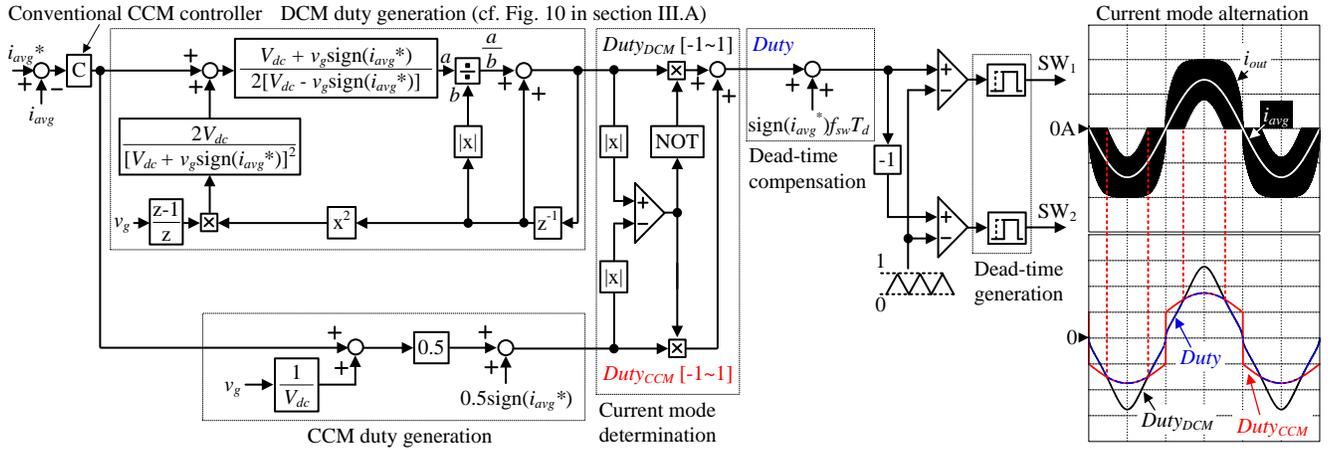
(c) Proposed inductance-independent CCM/DCM current control system with waveform of current mode alteration.
