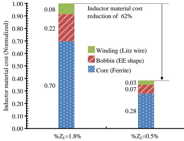
Fig. 21. Cost breakdown of inverter-side inductor material under two designs of  $\%Z_L$ . A cost reduction of 62% in the inductor material is achieved when decreasing the inverter-side inductor impedance from 1.8% to 0.5%. Note that the cost calculation is based on the actual price of the prototype components, and is normalized by the  $\%Z_L$  design of 1.8%.
