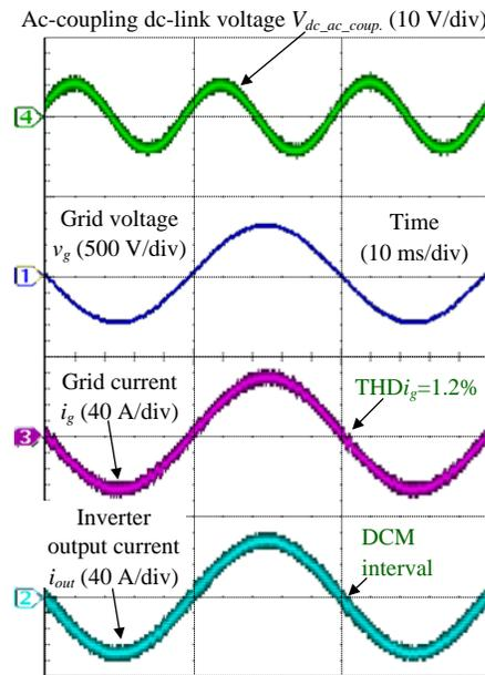
(c) Proposed CCM/DCM control,  $\%Z_L = 1.8\%$ , light load of 2 kW
