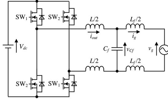
Fig. 1. Single-phase grid-tied inverter. An H-bridge inverter with a  $LCL$  filter is analyzed due to its simple configuration, which provides high fault-tolerant reliability. The inverter is operated under bipolar modulation and the impedance of each grid line is designed equally in order to minimize a common-mode current.
