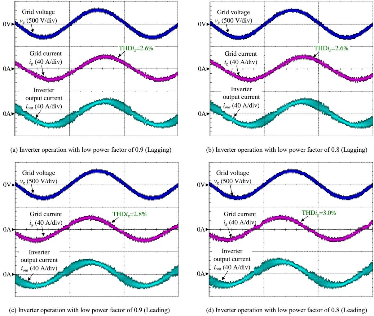
Fig. 18. Proposed CCM/DCM current control operation under low power factor with  $\%Z_L$  of 0.5%. When the grid variations occur, i.e. frequency instability or grid voltage sag, the grid-tied inverter is necessary to operate under a low power factor in order to avoid more serious events, e.g. power outage or voltage flickering.
