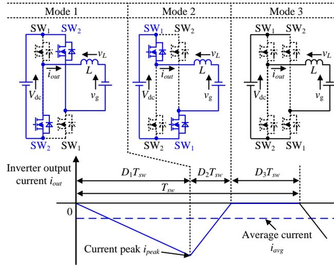
Fig. 9. Current path and inverter output current waveform in DCM when the grid voltage is negative. The same analysis procedure when the grid voltage is positive can be applied with the negative grid voltage.
