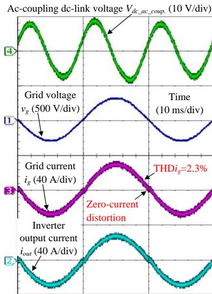
(a) Conventional CCM control,  $\%Z_L=1.8\%$ , rated load of 4 kW
