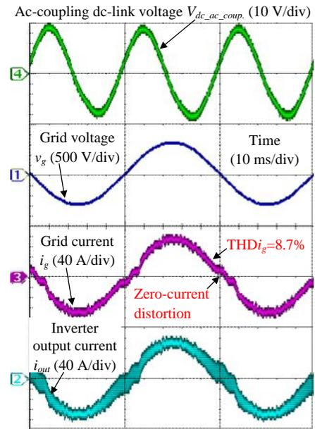
(b) Conventional CCM control,  $\%Z_L=0.5\%$ , rated load of 4 kW
