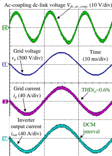
(a) Proposed CCM/DCM control,  $\%Z_L = 1.8\%$ , rated load of 4 kW
