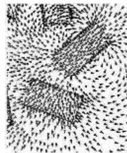
Fig. 4 Vector diagram of magnetic flux density at \theta = 40 deg.
