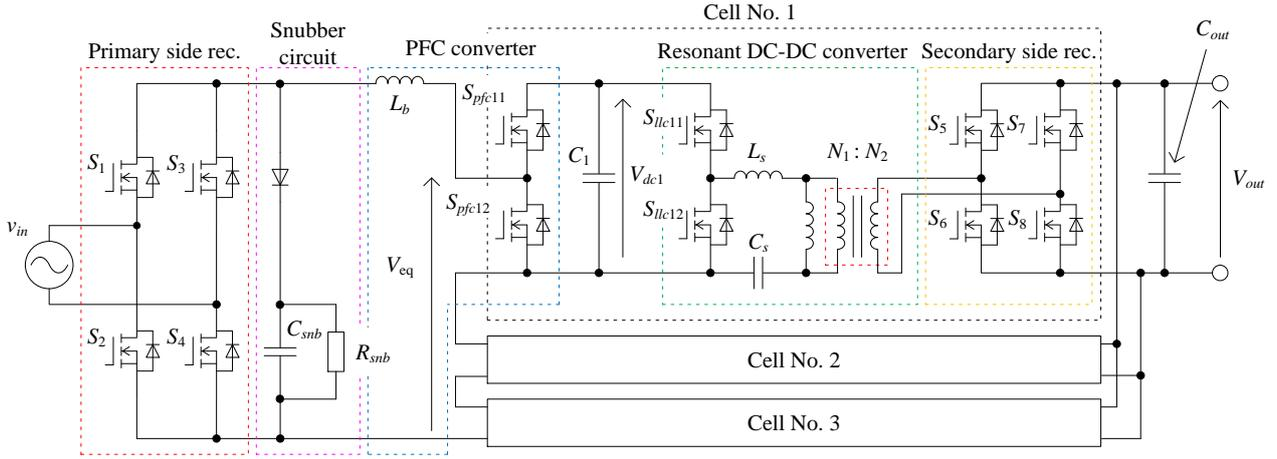
Fig. 1. Circuit configuration of proposed bidirectional single-phase SST.
