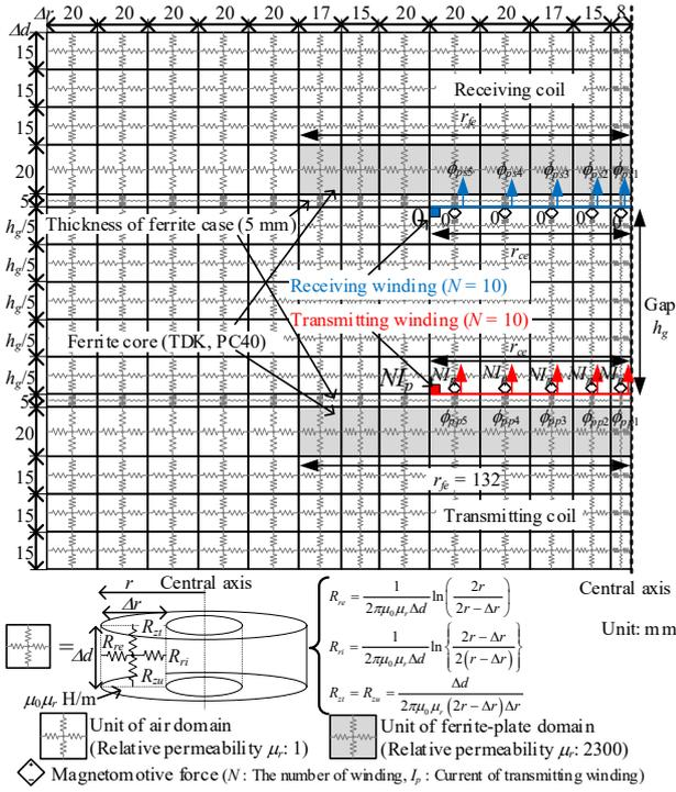
Fig. 1. Representative example of RNA model ( $r_{ce} = 80$  mm).
