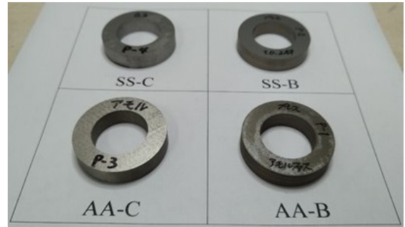
Fig. 1. Photograph of ring-cores made with the processing method as shown in Table 1.
