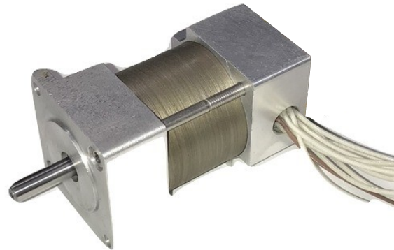
Fig. 4. Photograph of 70W-SRM made of blanked amorphous alloy foil.
