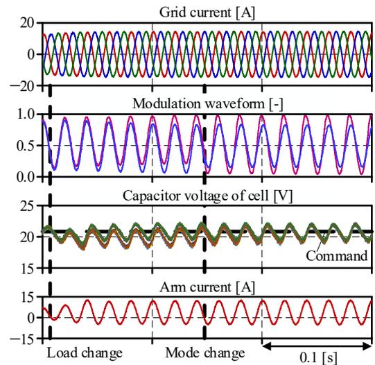
Fig. 11. Experimental result of transient behavior with proposed method under load change.
