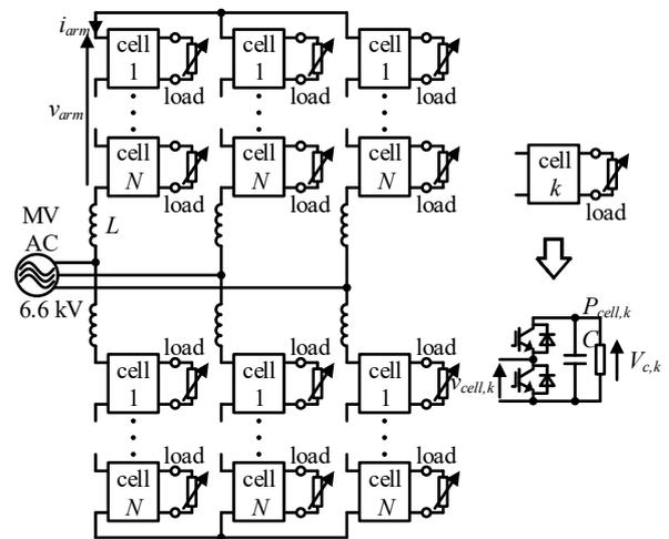
Fig. 1. Concept of multiport converter based on MMC.
