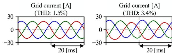
(b) Grid current when the proposed controller is applied. (c) Grid current 0.36 s after the controller change.
