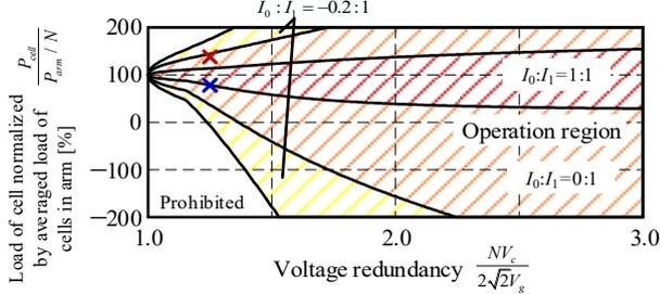
(c) With grid frequency compensation voltage (mode 2) and  $\phi_i^* = \pi/6$ . The maximum and the minimum load imbalance for the following simulation and experimental conditions (Fig. 8 and Fig. 12) are indicated.
