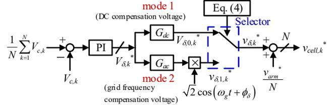
Fig. 3. Proposed intra-arm balance controller.
