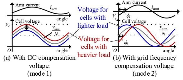
Fig. 5. Example of cell voltages with proposed intra-arm balance control under imbalanced load in one arm.
