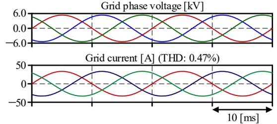
(a) Grid phase voltage and grid current.
