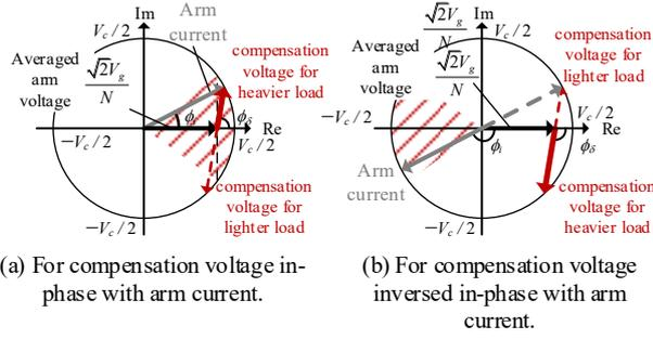
Fig. 4. Phasor diagram of grid frequency component of reference waveform  $\sin(\omega_g t + \phi_s)$ .
