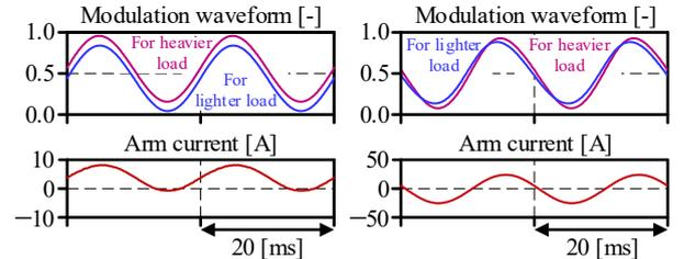
(b) Modulation waveforms for cells with DC compensation voltage (mode 1).
