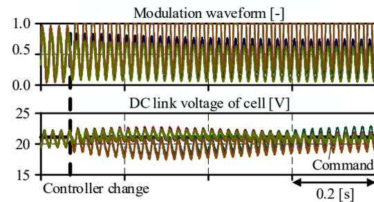
(a) Transient behavior of modulation waveform and DC link voltage of cells under converter change from proposed controller to conventional controller.
