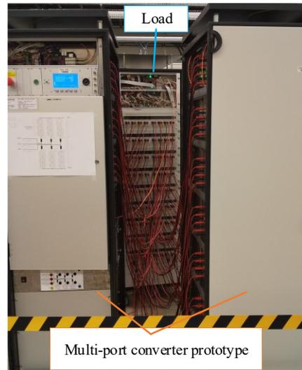
Fig. 9. The experimental setup of multiport converter prototype.
