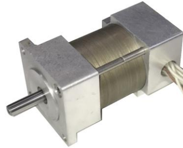
Fig. 2. Photograph of 70W-SRM made of blanked amorphous alloy foil.
