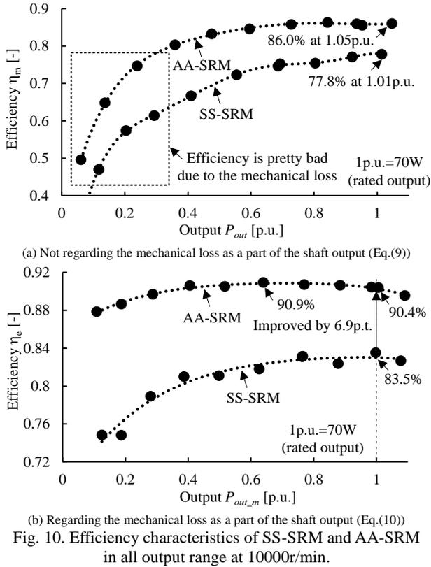
Fig. 10. Efficiency characteristics of SS-SRM and AA-SRM in all output range at 10000r/min.
