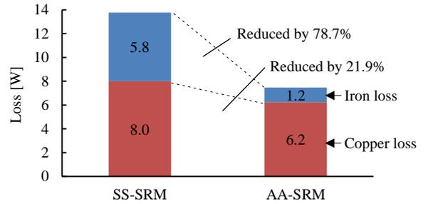
Fig. 12. Motor loss comparison between SS-SRM and AA-SRM of rated power (70W) at 10000r/min.
