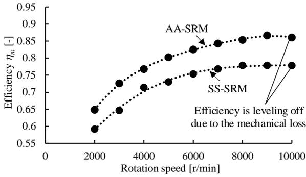
(a) Not regarding the mechanical loss as a part of the shaft output (Eq.(9))
