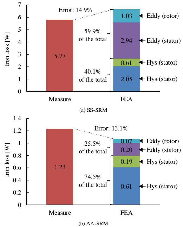
Fig. 16. Iron loss separation results of rated power (70W) at 10000r/min.
