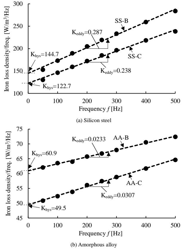
Fig. 4. Measured iron loss characteristics at 1.0T.
