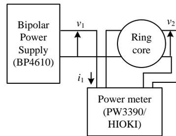
Fig. 2. Diagrams of measurement setup for ring-core
