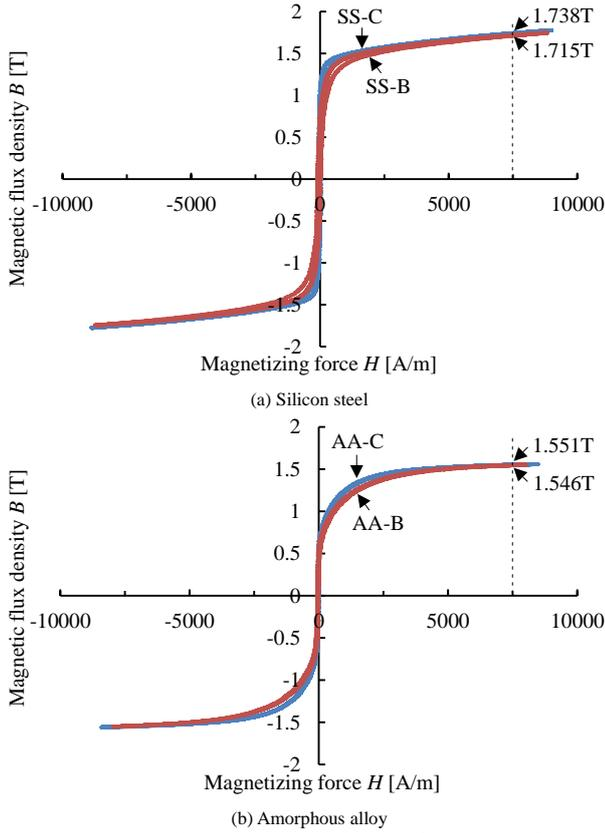
Fig. 3. Measured B-H characteristics at a frequency of 50Hz.
