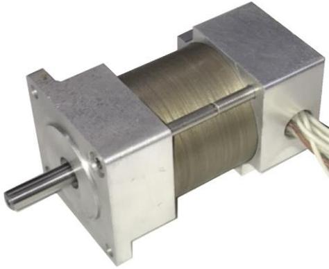
Fig. 6. Photograph of 70W-SRM made of blanked amorphous alloy foil.
