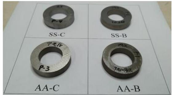
Fig. 1. Photograph of ring-cores made with the processing methods as shown in Table 1.
