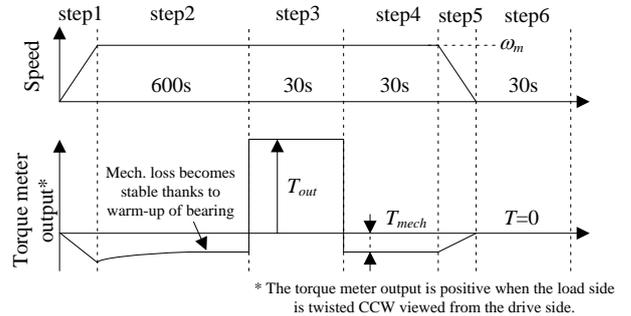
Fig. 9. The speed and the torque meter output during the experiment (Step1~Step6)
