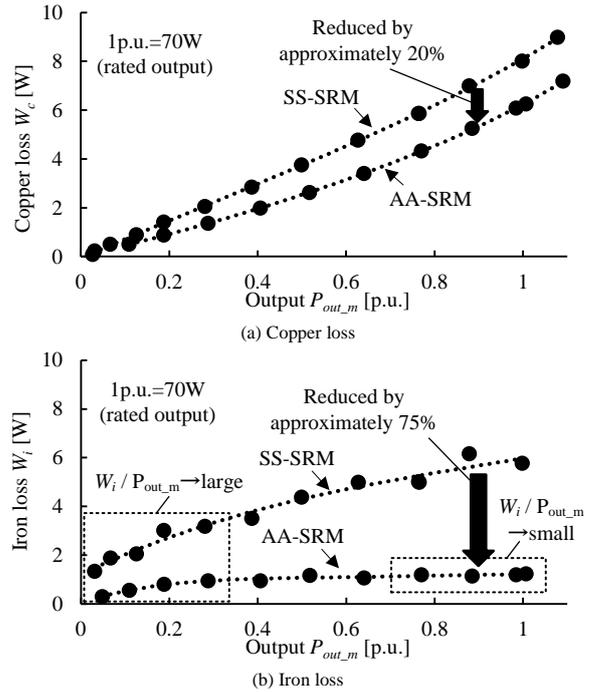
Fig. 11. Motor loss comparison between SS-SRM and AA-SRM in all output range at 10000r/min.
