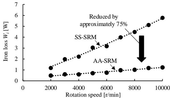
Fig. 14. Iron loss characteristics of SS-SRM and AA-SRM in all speed range at 1p.u. torque.
