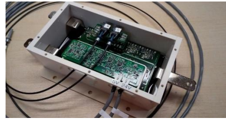
Fig. 12 Photograph of developed power module.
